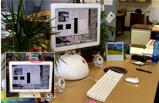
Figure 4: Ambient Gesture (AG) system available for interaction at the desktop. Inset shows position of standard web cam used in AG. Screen shows user training the system (as per Figure 3).
