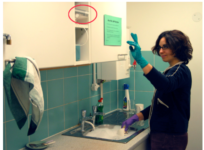
Figure 1: Ambient Gestures supports ‘in the environment’ system interaction so that users do not have to change their current task context in order to operate a computer application. Here, while washing up, gestures to the camera (circled in red) control a music browsing software application.
