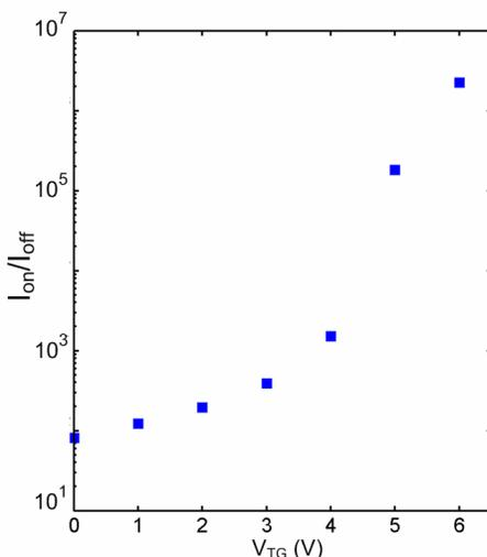
**Figure. 6.14.** The variation of the on/off current ratio in the simulated 200nm-thick dual gate OFET with the Top Gate voltage ( $V_{DS}=-0.5V$ ).
