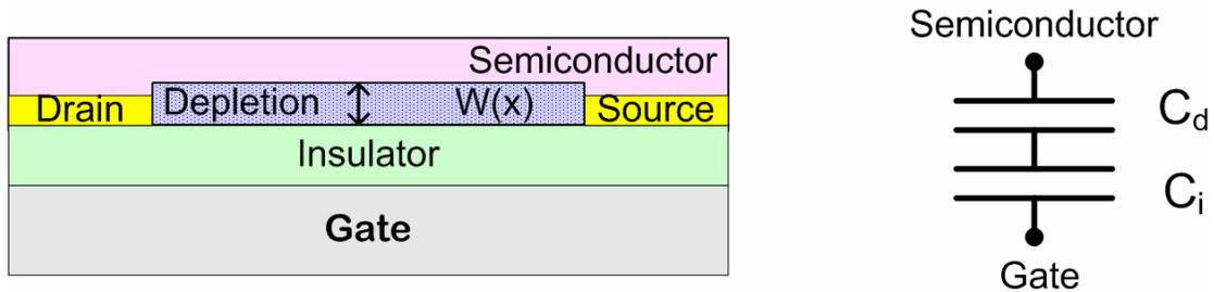
**Figure 5.2.** A schematic of the depletion layer in the OFET when  $V_{DS}=0$  V and the capacitive model of the transistor in the depletion mode.
