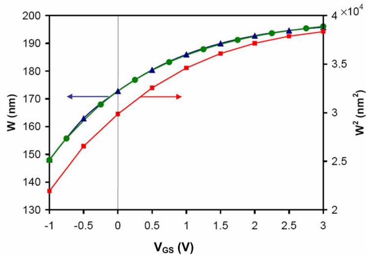
**Figure 5.11.** The depletion width versus the voltage. (▲) calculated  $W$  from the measured drain current (●) fit curve calculated from equation 5.15, (■)  $W^2$  versus the voltage.
