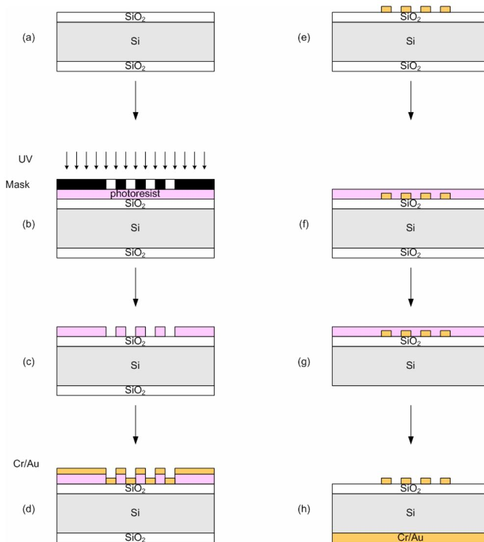
**Figure C.1.** Micro-electrode fabrication steps: (a) SiO<sub>2</sub>/Si/SiO<sub>2</sub> wafer (b) photolithography (c) developing (d) metal deposition (e) lift-off (f) photoresist coating (g) SiO<sub>2</sub> back side etching (h) the backside electrode deposition.
