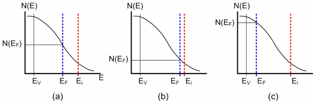
**Figure 2.8.** (a) Density of states and position of the Fermi level in a hypothetical doped p-type organic semiconductor. Carrier density and mobility (b) reduce or (c) increase when the Fermi level changes.
