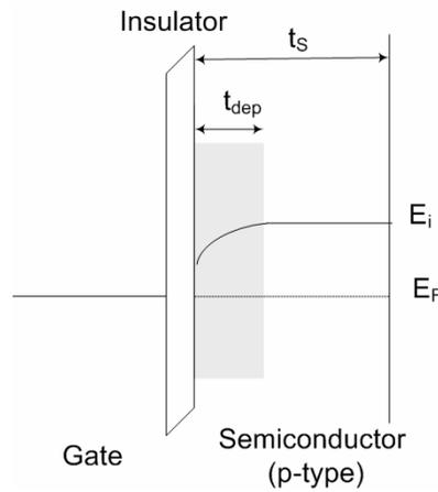
**Figure. 6.2.** The energy diagram for a MIS device at the equilibrium ( $V_{GS}=0$ ).
