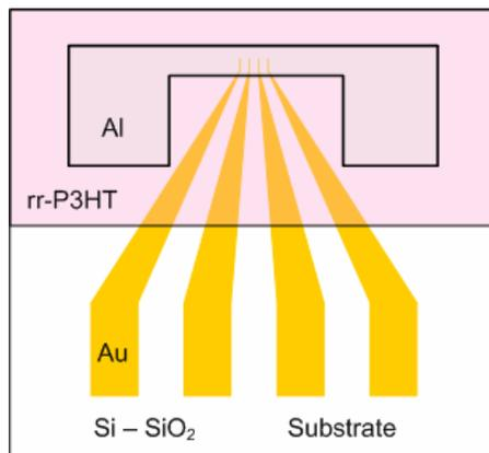
**Figure 4.4.** A schematic of the top view of the sample after the aluminium deposition.
