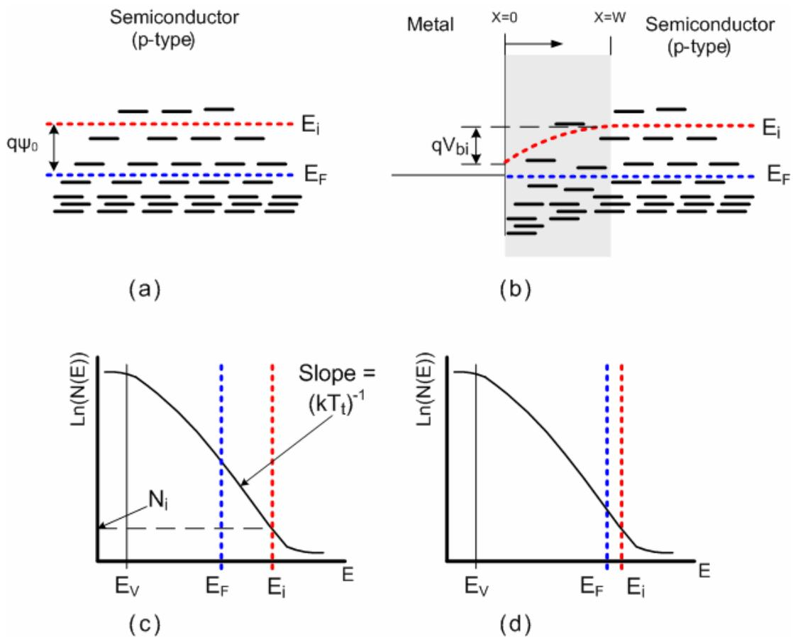
**Figure 4.2.** The Fermi level in the organic semiconductor (a) before and (b) after a metal junction is formed. The density of states in the organic semiconductor with an exponential tail states and the position of the Fermi level at the surface of the semiconductor (c) before and (d) after the junction.
