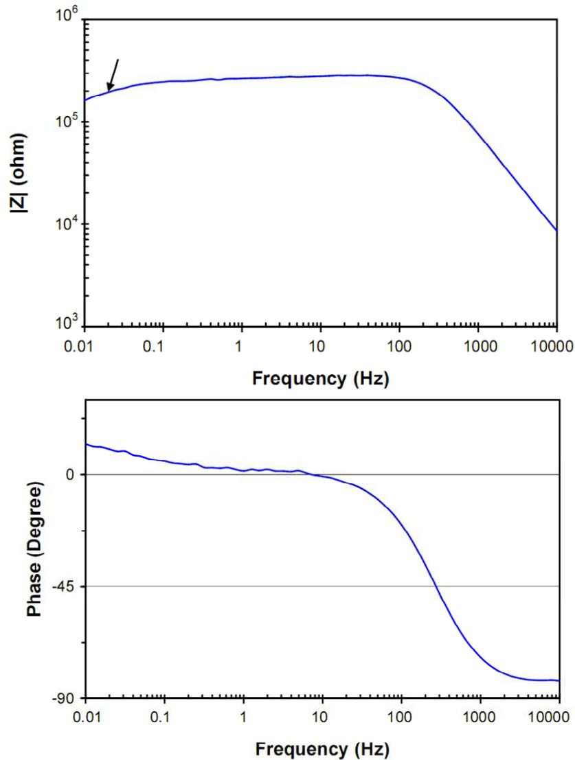
**Figure 4.24.** The magnitude and phase of small signal impedance of the organic Schottky diode at 7 V DC bias.
