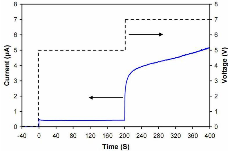
**Figure 4.25.** The organic Schottky diode current in response to a voltage pulse.
