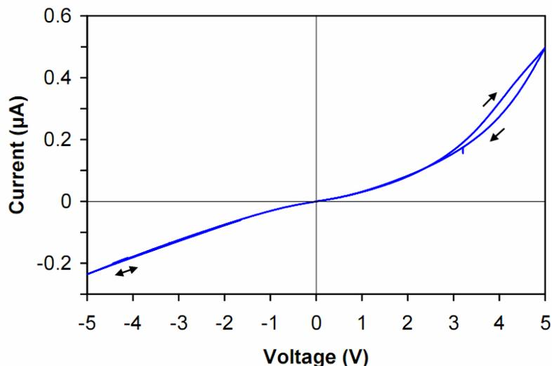
**Figure 4.21.** The  $I$ - $V$  characteristic of the organic Schottky diode in the range of  $\pm 5\text{V}$  showing a capacitive hysteresis loop.
