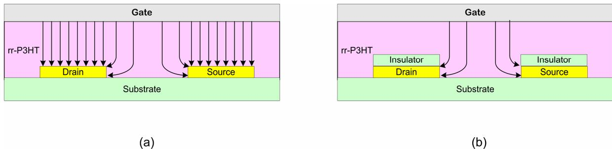
**Figure 5.14.** (a) The gate current paths in the experimental OMESFET (b) the solution to reduce the gate current. ( $V_{GS} > 0$  and  $V_{DS} = 0$ )
