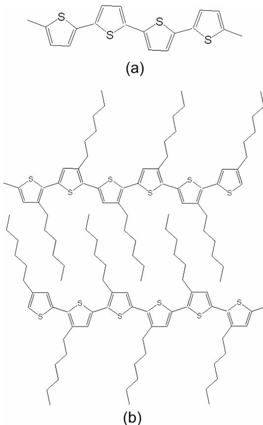
**Figure 2.4.** (a) Chemical structure of polythiophene (b) rr-P3HT with an interdigitated molecular structure.
