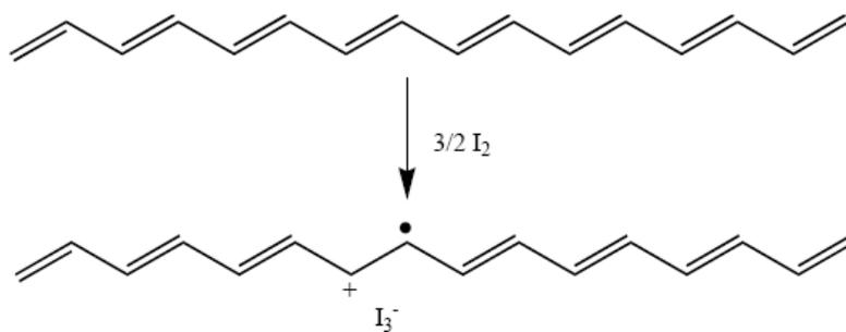
**Figure 2.3.** Generation of a hole in polyacetylene by oxidizing the polymer. The iodine acts as a dopant for the polymer.
