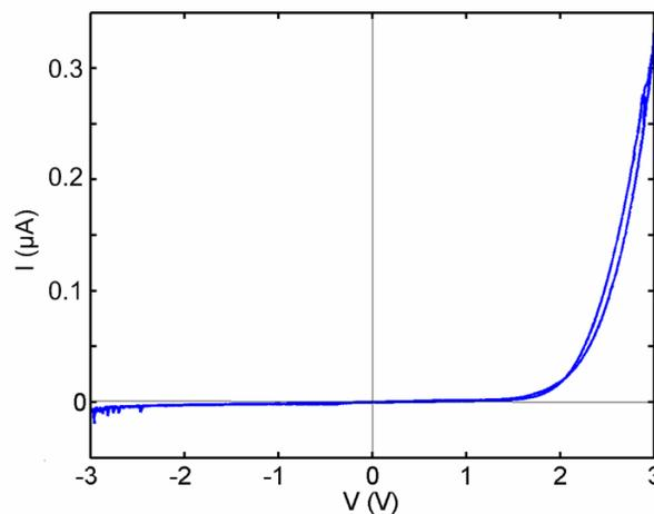
**Figure 4.9.** The I-V characteristics of an Al/rr-P3HT/Au Schottky diode made and tested in air.
