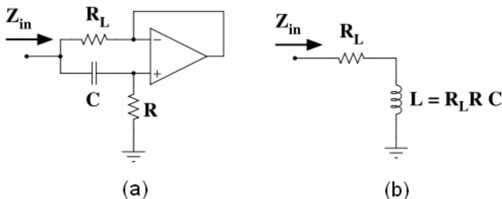
**Figure 4.27.** (a) Simulation of an RL circuit using positive feedback in the op-amp and (b) its equivalent circuit.
