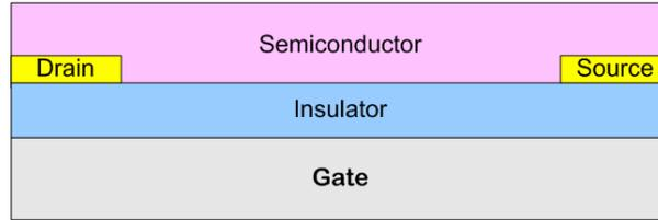
**Figure 5.1.** A schematic of a bottom-contact OFET.
