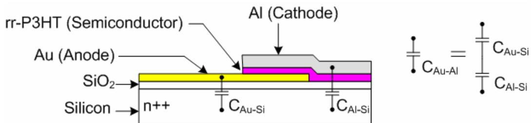
**Figure 4.18.** The parasitic capacitance between the gold and the aluminium electrodes. The gold/silicon capacitance ( $C_{\text{Au-Si}}$ ) is in series with the capacitance between the aluminium layer and the silicon ( $C_{\text{Al-Si}}$ ).
