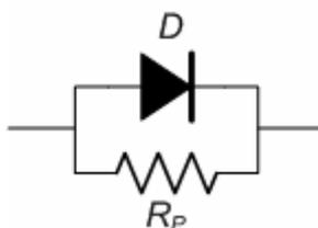
**Figure 4.12.** The proposed model for the organic Schottky diode.
