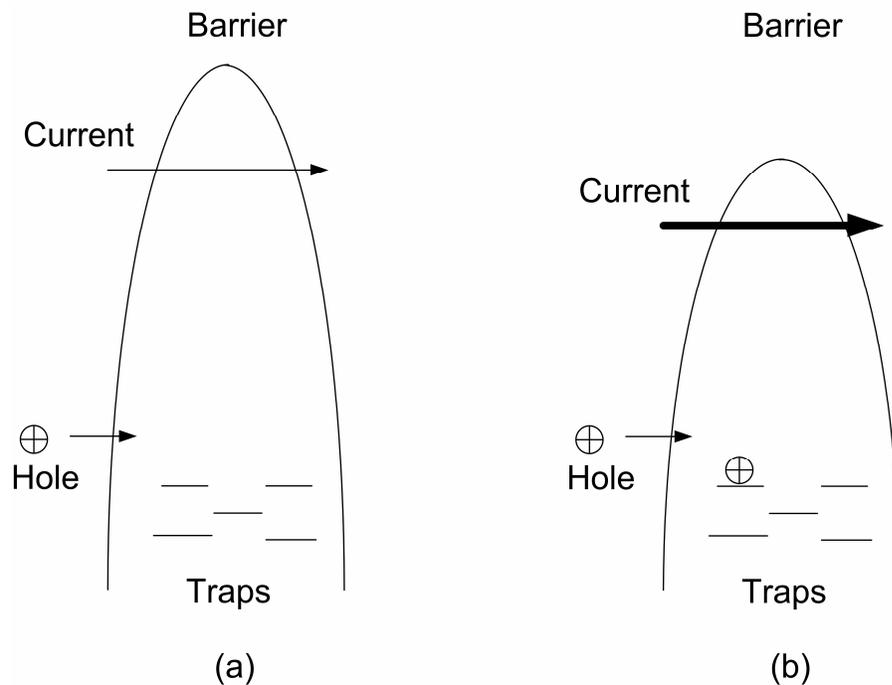
**Figure 4.26.** (a) The barrier of the middle layer limits the current in the Schottky diode. (b) Trapped charge reduces the barrier and increases the current.
