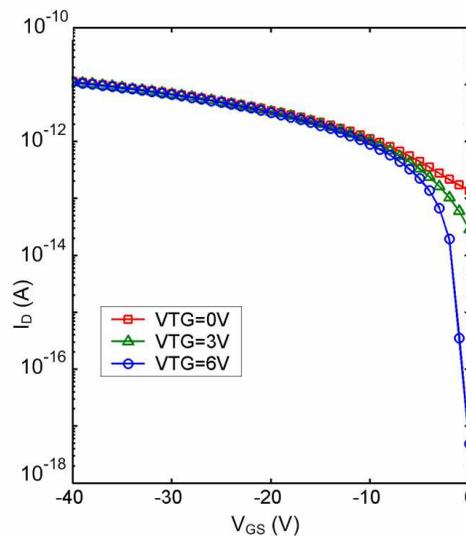
**Figure. 6.10.** The transverse characteristics of the simulated 200 nm dual gate OFET at different Top Gate biases ( $V_{DS}=-0.5V$ ).
