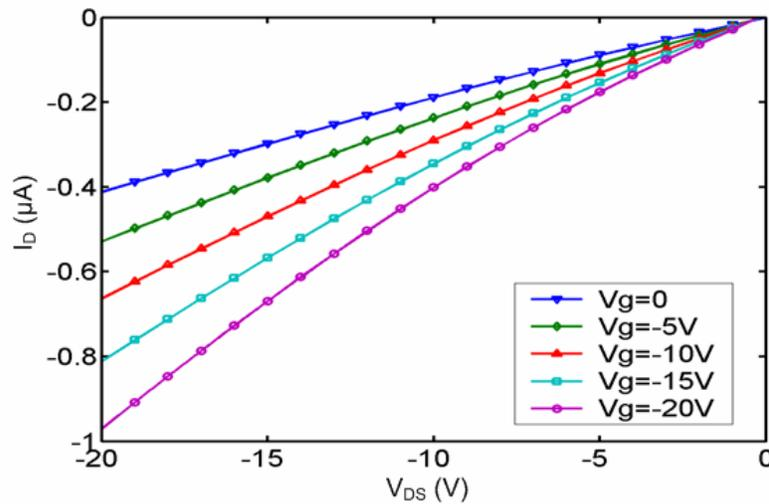
**Figure 5.8.** The output characteristic of the OFET with the polymer thickness of 200 nm.
