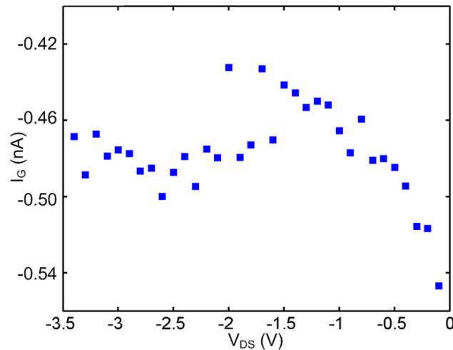
**Figure 5.12.** The gate current versus the drain source voltage in the OMESFET ( $V_{GS}=-1$  V).
