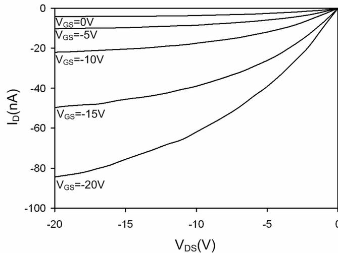
**Figure 6.16.** The output characteristics of an OFET following aluminium deposition over the semiconducting layer (Dual gate organic transistor).
