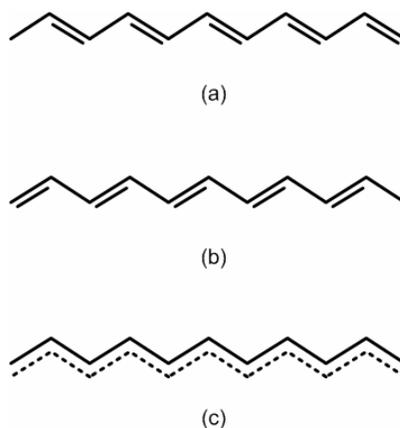
**Figure 2.2.** (a) (b) Degenerate forms of polyacetylene. (c) Delocalized electrons all along the polyacetylene back bone instead of the conjugated double bonds.
