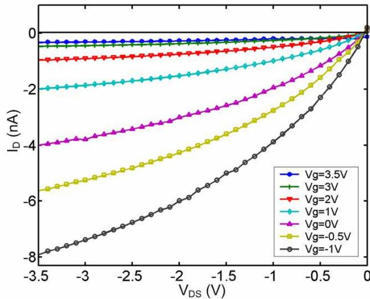
**Figure 5.9.** The measured output characteristic of the OMESFET.
