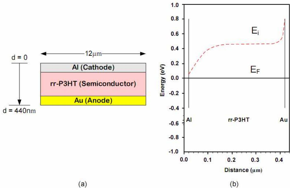
**Figure 4.3.** (a) The schematic of the simulated organic Schottky diode and (b) the energy diagram at equilibrium.
