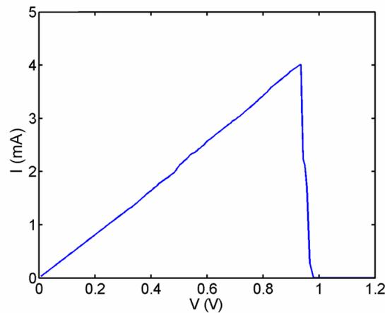
**Figure 4.7.** The  $I$ - $V$  curve of a diode with a high rate deposition of aluminium showing the short circuit and burning the shorted paths at high voltages.
