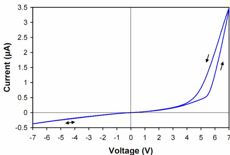
**Figure 4.22.** The  $I$ - $V$  characteristic of the organic Schottky diode in the range of  $\pm 7\text{V}$  showing an inductive hysteresis loop.
