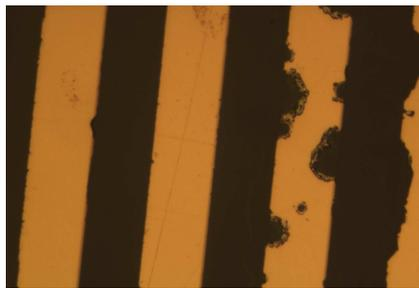
**Figure 4.8.** The optical image of a damaged micro electrode after the burning of the conductive paths in a Schottky diode.
