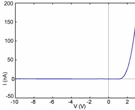
**Figure 4.15.** The  $I$ - $V$  characteristic of an organic Schottky diode made in the glove box.
