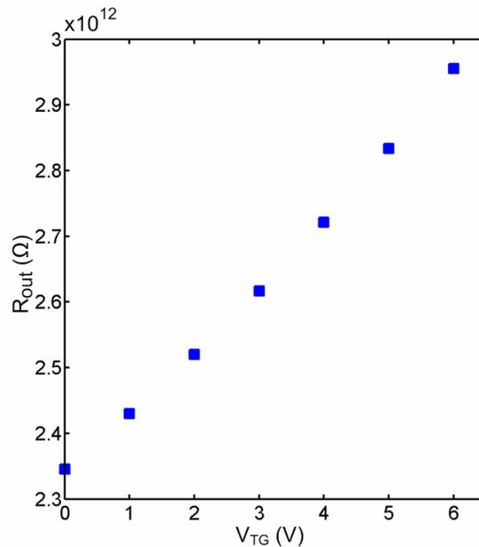
**Figure. 6.13.** The variation of the output resistance in the simulated 200 nm-thick dual gate OFET with the Top Gate voltage ( $-60 < V_{DS} < -40$  V and  $V_{GS} = -40$  V).
