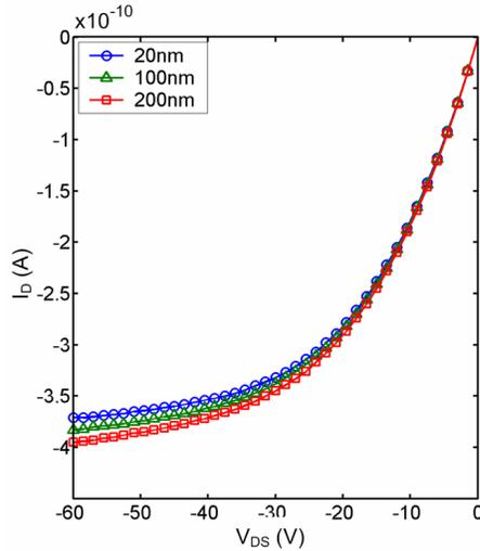
**Figure. 6.6.** The output characteristics of the simulated OFETs with the different semiconductor thicknesses ( $V_{GS}=-40V$ ).
