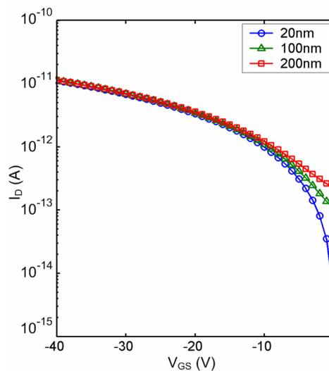
**Figure. 6.4.** The transverse characteristics of the simulated OFETs with the different semiconductor thicknesses ( $V_{DS}=-0.5\text{V}$ ).
