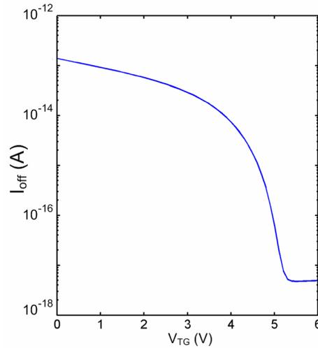
**Figure. 6.9.** The variation of the off current in the simulated 200 nm-thick dual gate OFET with the Top Gate voltage ( $V_{DS}=-0.5V$  and  $V_{GS}=0V$ ).
