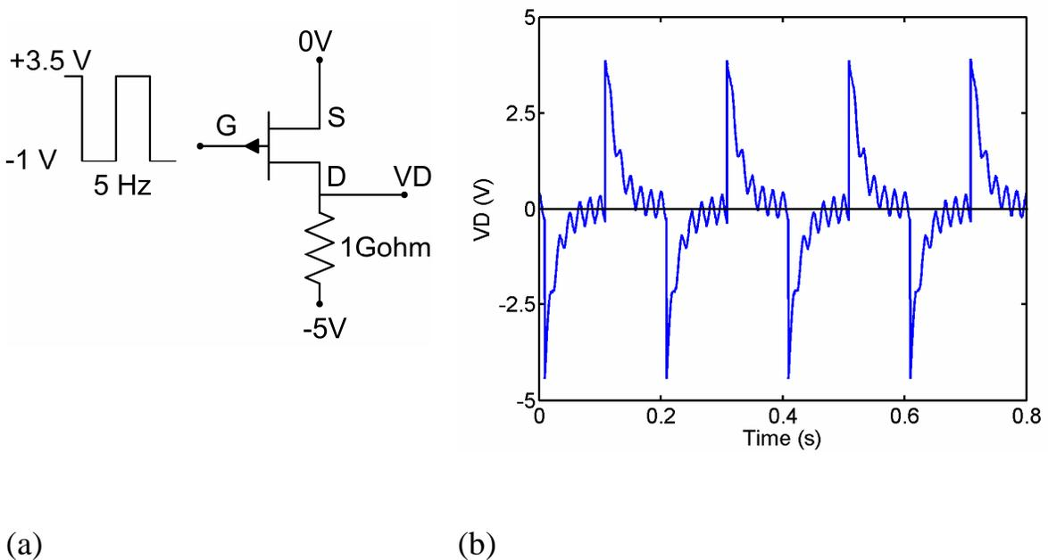
**Figure 5.13.** (a) The circuit diagram applied to monitor the switching properties of the OMESFET and (b) the AC pulse response of the OMESFET.
