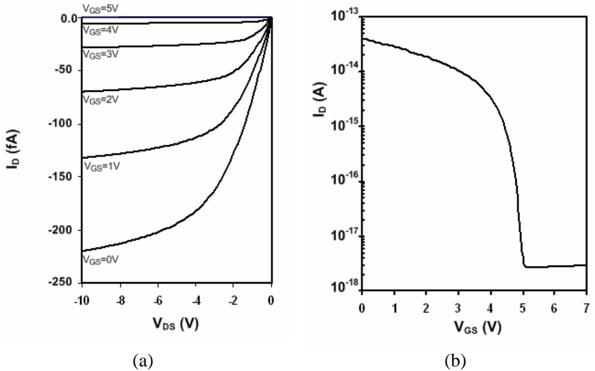
**Figure 5.5.** (a) The output and (b) transfer characteristics ( $V_{DS}=-0.5V$ ) of the simulated OMESFET with a channel width of  $1\mu m$  and a length of  $4\mu m$ .
