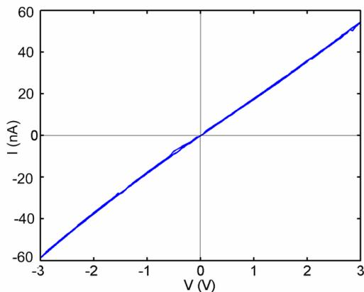
**Figure 4.5.** The  $I$ - $V$  curve between two adjacent gold electrodes in a sample with 200 nm thick rr-P3HT and no aluminium layer.
