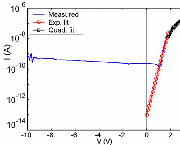
**Figure 4.16.** The  $I$ - $V$  characteristic of the diode in a semi-log plot. The red line ( $\circ$ ) is an exponential fit in the forward bias and the black ( $\square$ ) line indicates the quadratic function describing the SCLC. The red and black lines form good fits, hiding the experimental data above 1.1 V.
