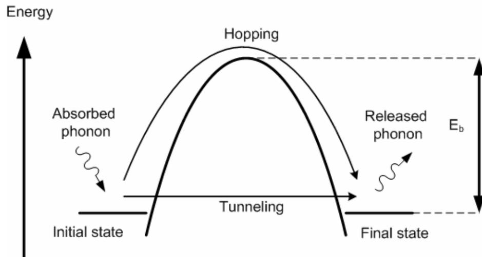
**Figure 2.7.** Hopping versus tunneling between two localized states.
