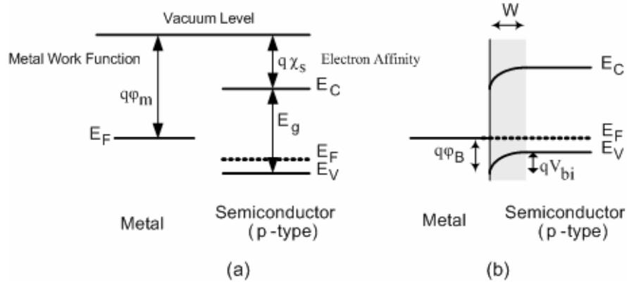
**Figure 4.1.** The energy diagram of a metal and a semiconductor (a) before and (b) after the junction.
