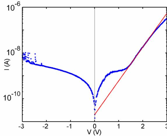
**Figure 4.10.** The  $I$ - $V$  curve in a semi-log plot. The red (straight) line is a fit curve to the exponential part of the current.
