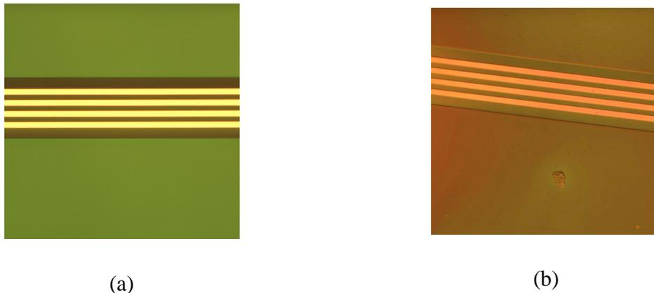
**Figure 4.6.** Optical microscope image of the micro electrode (a) before and (b) after the polymer deposition (the width of each electrode is 4  $\mu\text{m}$ ).
