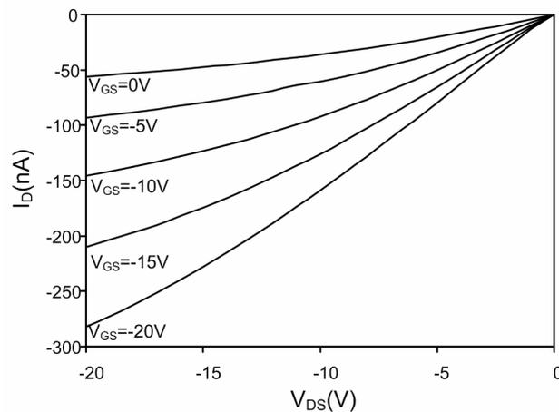
**Figure 6.15.** The measured output characteristics of a thick-film OFET.
