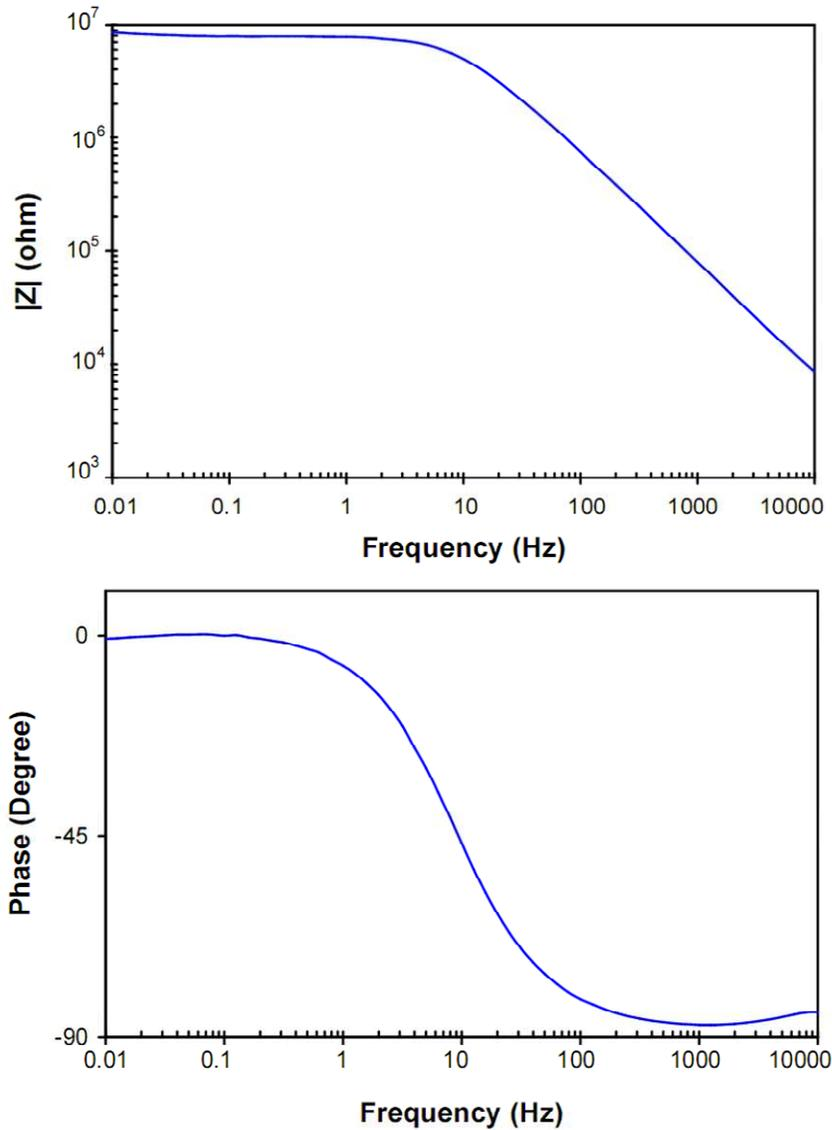
**Figure 4.23.** The magnitude and phase of small signal impedance of the organic Schottky diode at 4V DC bias.
