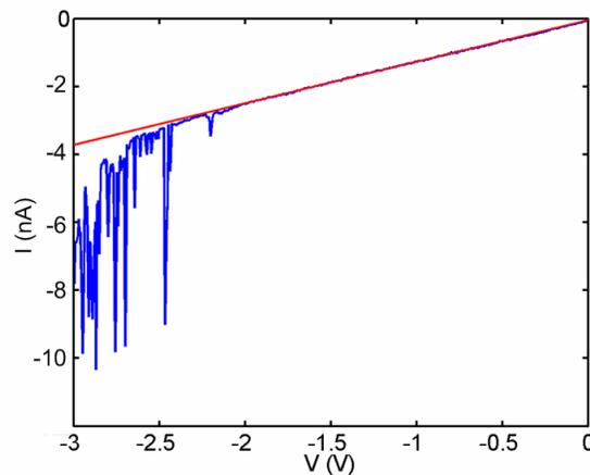
**Figure 4.11.** The reverse bias characteristic of the diode. The red (straight) line is a fit curve to the current.
