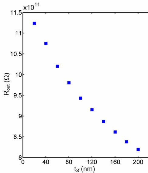
**Figure. 6.7.** The variation of the output resistance in the simulated OFETs with the semiconductor thickness ( $-60 V < V_{DS} < -40 V$  and  $V_{GS}=-40 V$ ).
