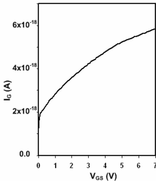
**Figure 5.7.** The input characteristic of the simulated OMESFET.
