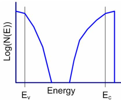
**Figure 2.6.** The density of states (DOS) in a semilog plot for a hypothetical amorphous semiconductor.
