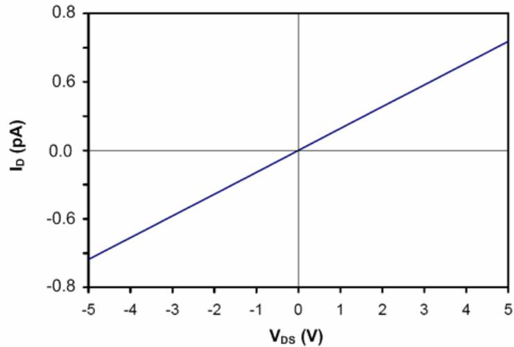
**Figure 5.6.** The simulated I-V curve between the drain and source terminals of the OMESFET in the absence of the gate contact. The slope indicates  $G_0$  in the OMESFET.
