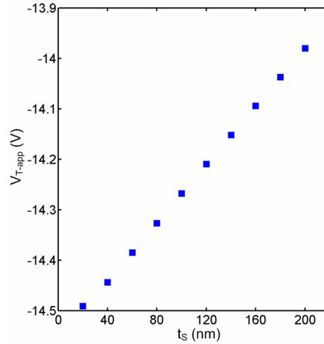
**Figure. 6.5.** The variation of  $V_{Tapp}$  in the simulated OFETs with the semiconductor thickness ( $V_{DS}=-0.5V$ ).
