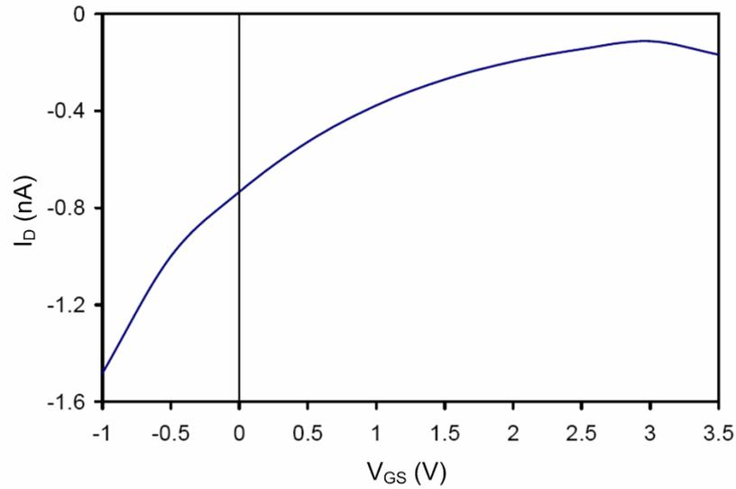
**Figure 5.10.** The measured  $I_D$ - $V_{GS}$  characteristics of the OMESFET at  $V_{DS}=-0.3V$ .
