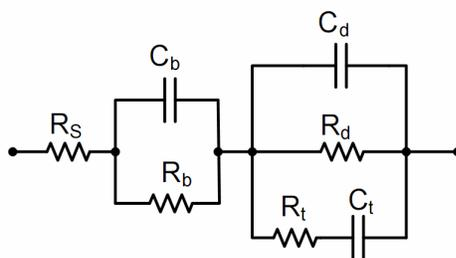
**Figure 4.20.** AC model of an organic Schottky diode.
