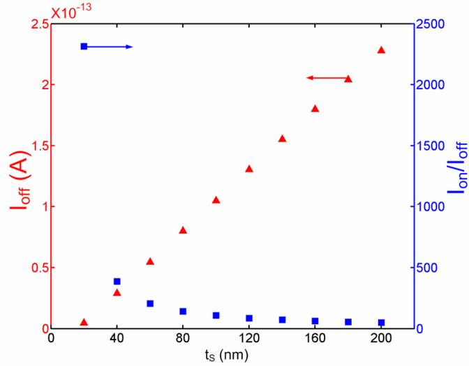
**Figure. 6.8.** The variation of the off current and the on/off current ratio in the simulated OFETs with the semiconductor thickness ( $V_{DS}=-0.5V$ ).
