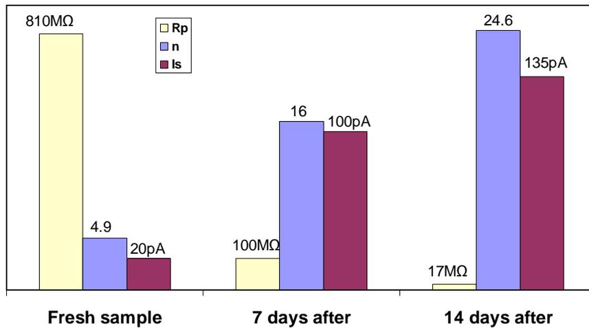
**Figure 4.13.** The drift of the diode parameters with time in two weeks.
