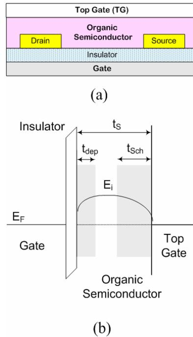
**Figure. 6.3.** (a) A schematic of a dual gate OFET and (b) the energy diagram at the both gate interfaces (equilibrium condition –  $V_{GS} = V_{TG} = 0V$ ).
