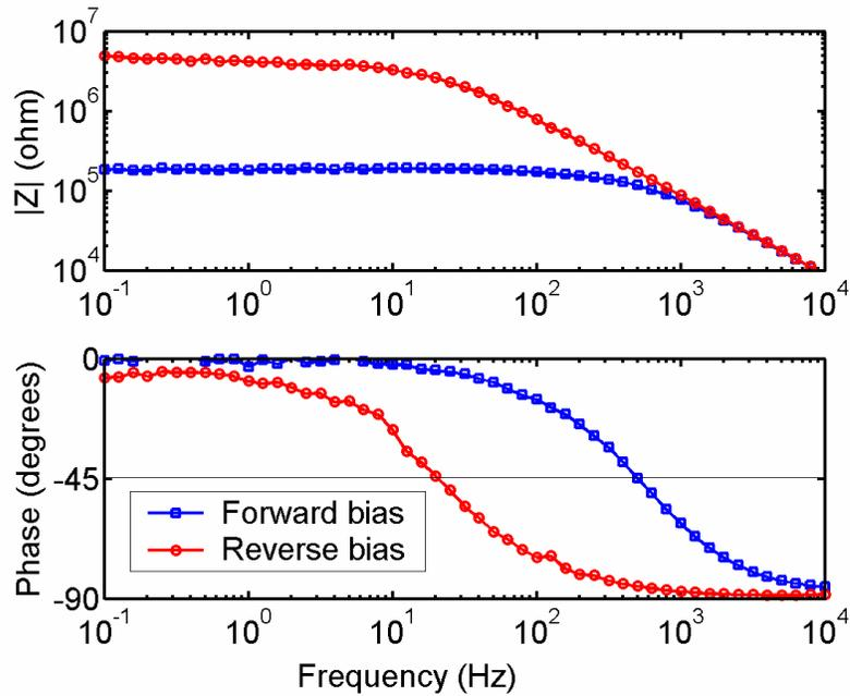
**Figure 4.17.** The Bode plot of the impedance in an organic Schottky diode. The blue and red curves are the impedances in the forward bias (2V) and the reverse bias (-2V), respectively.
