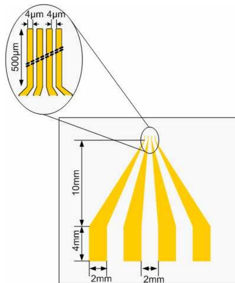
**Figure 3.1.** The micro-electrode designed for organic electronic devices.
