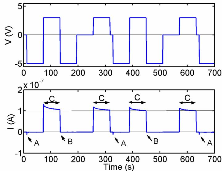
**Figure 4.19.** The applied voltage to the organic Schottky diode and its current response.
