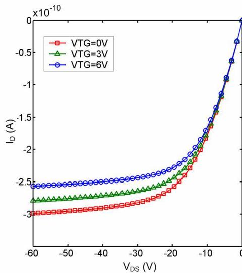
**Figure. 6.12.** The output characteristics of the simulated 200nm dual gate OFET in different biases of the Top Gate ( $V_{GS}=-40V$ ).
