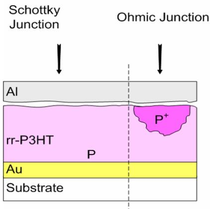
**Figure 4.14.** Non-uniform junction between the organic semiconductor and aluminium.
