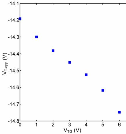
**Figure. 6.11.** The variation of the apparent threshold voltage in the simulated 200nm-thick dual gate OFET with the Top Gate voltage ( $V_{DS}=-0.5V$  and  $V_{GS}=-40V$ ).
