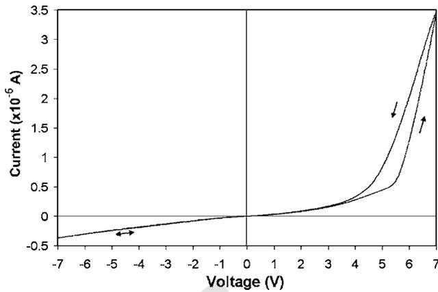
FIG. 4. Current-voltage ( $I$ - $V$ ) characteristic of the organic Schottky diode in the range of  $\pm 7$  V showing an inductive hysteresis loop.
