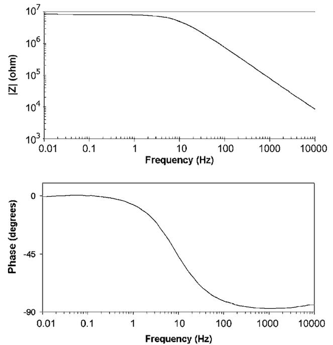
FIG. 5. The magnitude and phase of small signal impedance of the organic Schottky diode at 4 V dc bias.
