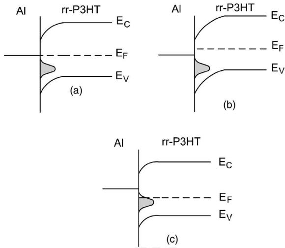
FIG. 8. The proposed band diagram of the Schottky junction between the aluminum and rr-P3HT with a Gaussian distribution of donorlike localized states (a) at equilibrium, (b) the reverse bias, and (c) the forward bias above the threshold. Impurities are neutralized in the (a) and (b), while the localized states located above the Fermi level are ionized in (c).
