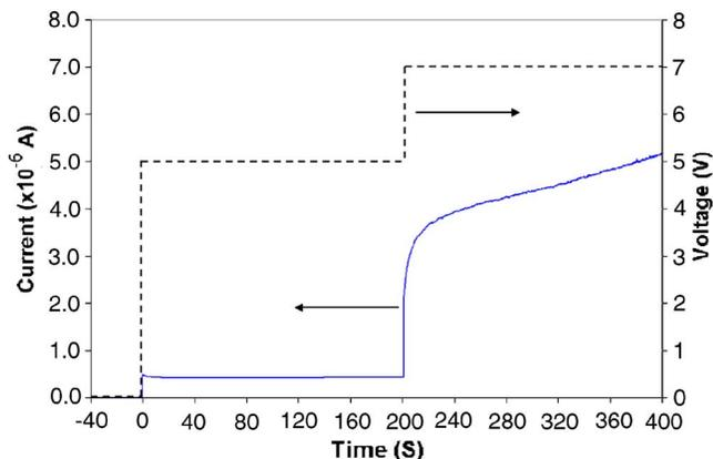
FIG. 7. The organic Schottky diode current in response to a voltage pulse.
