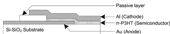
FIG. 2. The side view of the organic Schottky diode made of rr-P3HT (not to scale).
