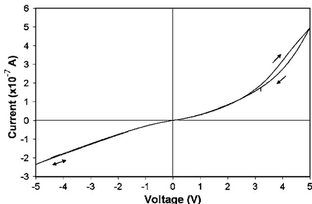
FIG. 3. Current-voltage ( $I$ - $V$ ) characteristic of the organic Schottky diode in the range of  $\pm 5$  V showing a capacitive hysteresis loop.
