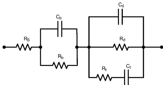
FIG. 1. ac model of an organic Schottky diode consisting of bulk capacitance and resistance ( $C_b$ - $R_b$ ), junction capacitance and resistance ( $C_d$ - $R_d$ ), trap associated capacitance and resistance ( $C_t$ - $R_t$ ) and the bulk semiconductor resistance  $R_S$ .
