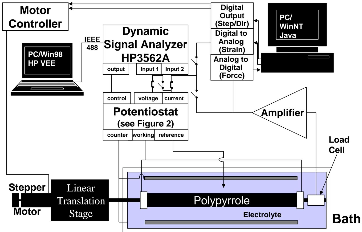
**Figure 1:** Diagram of the experimental apparatus for measuring polypyrrole admittance. Strain to current and stress to current are measured by switching connections to the DSA.
