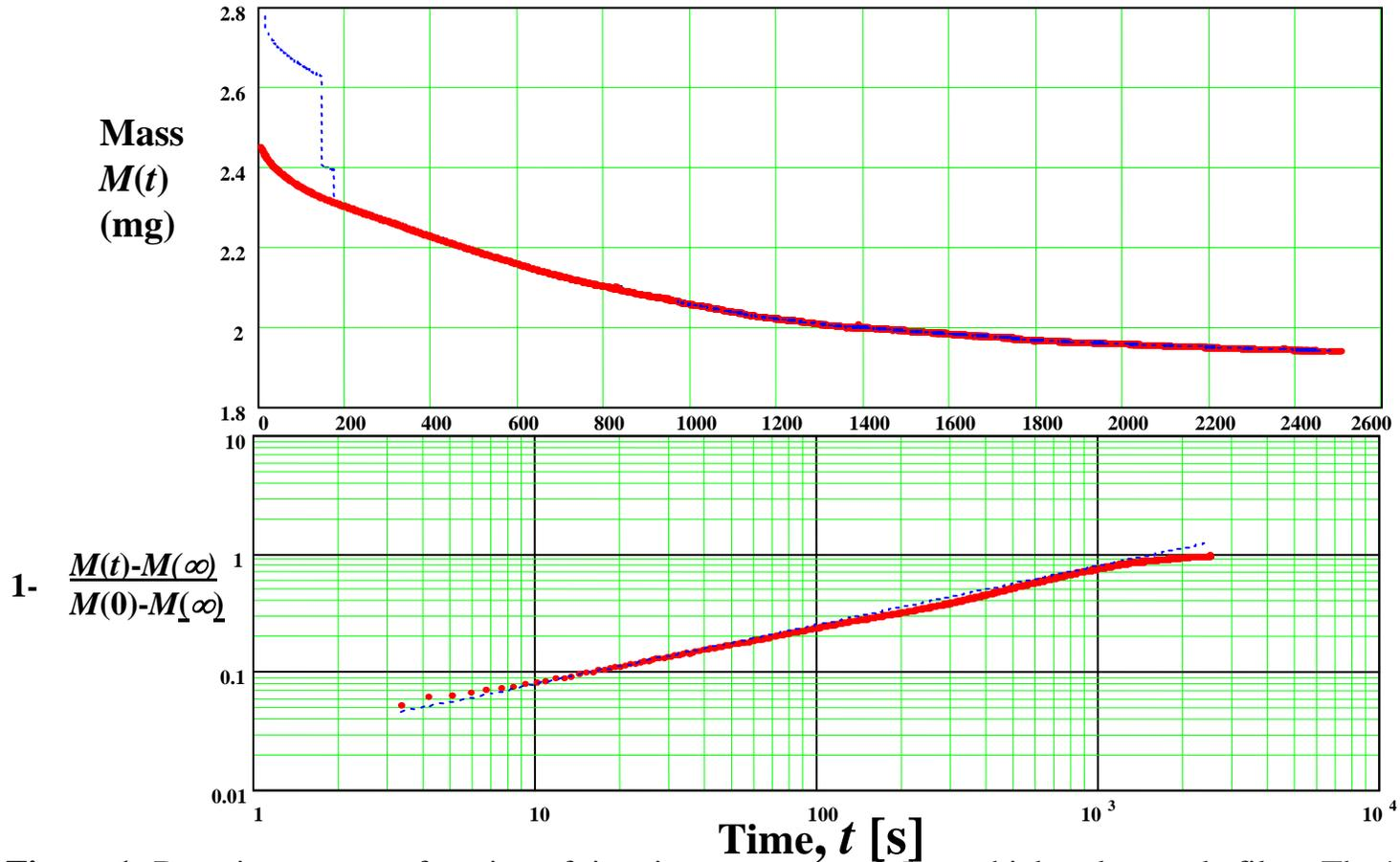
**Figure 1:** Drop in mass as a function of time in an as grown  $8.5 \mu\text{m}$  thick polypyrrole film. The  $\frac{1}{2}$  slope in the log-log plot at the bottom suggests that mass loss is diffusion limited. The blue points in the top figure show the actual measured mass loss, while the red line is the corrected mass loss, accounting for the dropping of two polymer flakes from the weighing pan.
