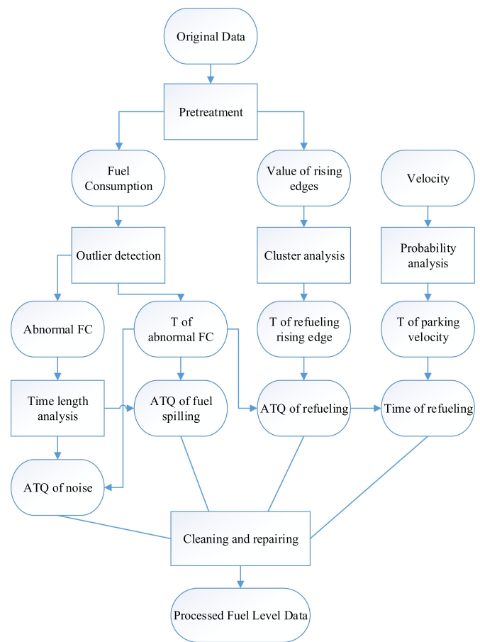
Fig. 11. Process of the cleaning and repairing method. (FC: fuel consumption; T: threshold; ATQ: abnormal time quantum).
