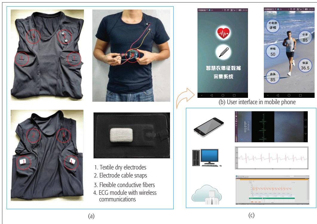
Figure 5. Wearable 2.0 testbed: a) ECG dry electrodes and signal acquisition module in the EPIC Wearable 2.0 testbed; b) three modes for body signal visualization: mobile phone, PC, and cloud.
