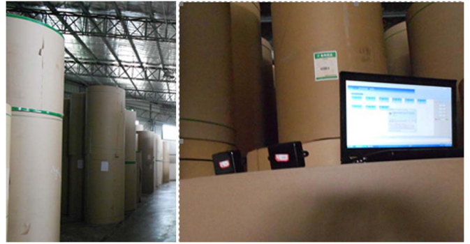
Fig. 9. Using the iLocate system in a carton packing plant that is 400 m × 300 m × 3 m. In this case, we have tested various passive RFID hardware, including Alien 9900+ readers and Impinj R420 readers. Their identification rates are less than 2% due to the severe signal shielding by many large paper pillars.
