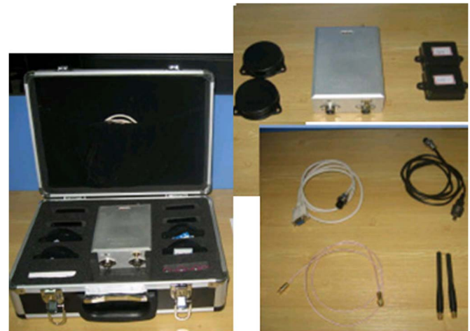
Fig. 7. Basic set of RTLS hardware for the iLocate system, which consists of a reader, two reference tags, six active tags, two antennas, and one universal serial bus, together with documents. An enriched toolbox contains RFID coordinators and an RFID deployment tool.
