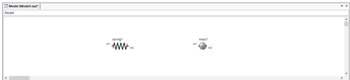
Fig. 7: Diagram view with two unconnected model elements ( Spring and Mass from the library Linear Mechanics )
