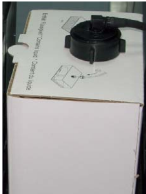
Figure 7-83: Waste container with drain tube attached
