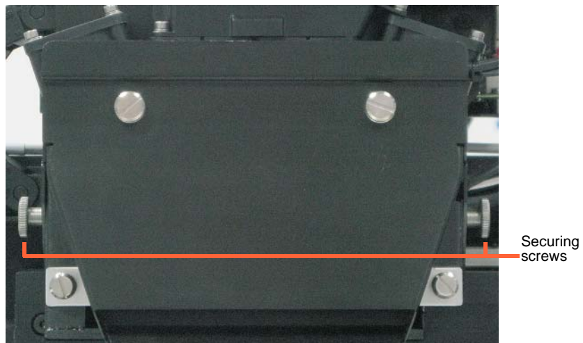
Figure 7-39: UV-lamp-assembly securing screws
