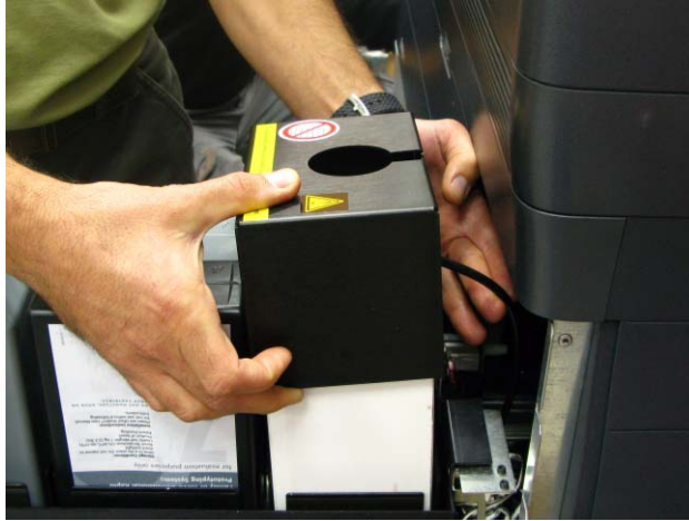
Figure 7-82: Removing the waste-container cover
