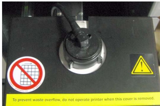
Figure 7-84: Fireproof cover installed over the waste container
