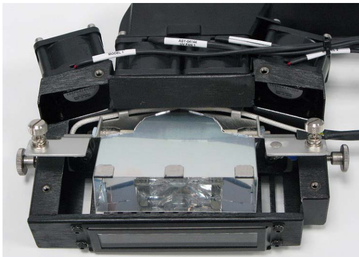
Figure 7-76: Removing the UV reflector from the UV assembly
