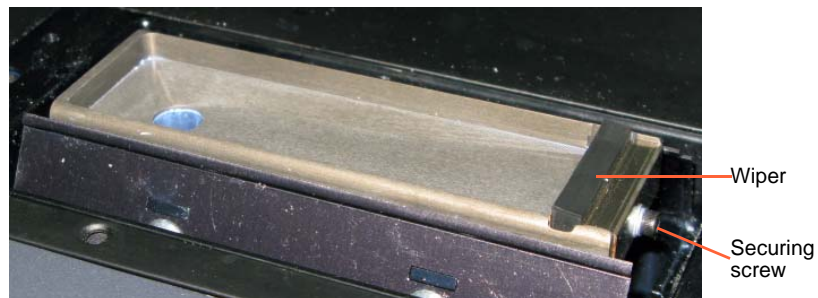
Figure 8: Wiper and excess-material drain
