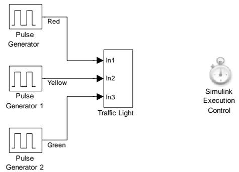
If you do not have the Real-Time execution control block loaded (see tools page), the stopwatch will not appear. Instead you will see a broken link. You can delete this block but the simulation will run faster than normal.
