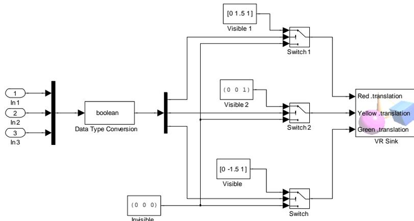
If a broken link appears instead of the VR Sink, open the block and make sure that the source file is correct and that the translation block is checked under the Red, Yellow and Green transforms.
