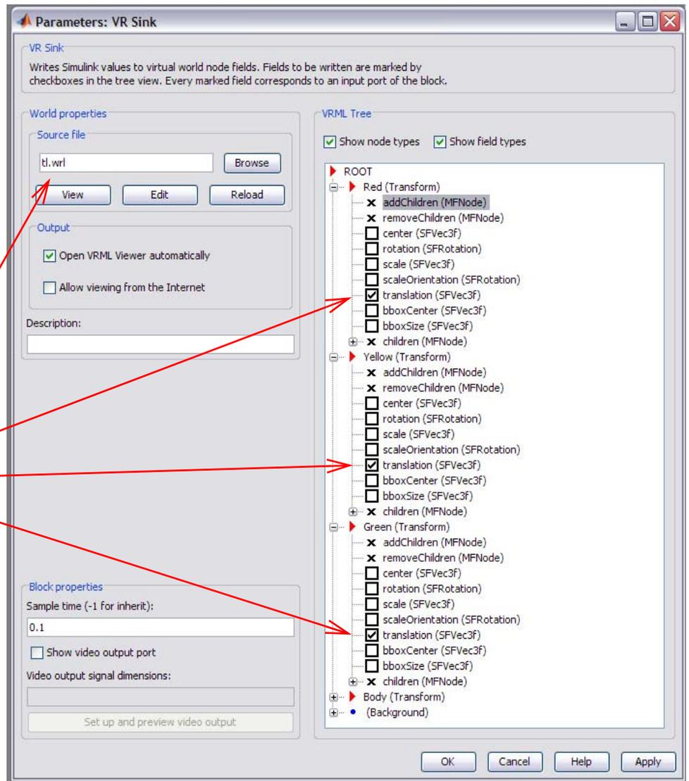
Run the simulation to make sure that you have it working properly. Double click the VR Sink block to see the graphic.
