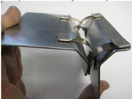
Nitinol is not weldable, but it can be spot welded between two layers of stainless steel:
