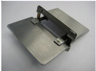
With strips made of Nitinol a 90 degree bend is easily achievable:
