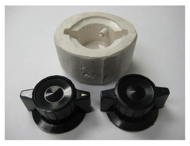
The most interesting applications of polymer replications are actually at the microscopic scale, where parts are too small to machine. The master can be done by micromachining techniques (photo-lithography etc) and many low cost copies can be made by replication. Life of a silicone mold is a few hundred parts. Mold should be baked at 200°-250° every 10-20 parts to drive off impurities.
