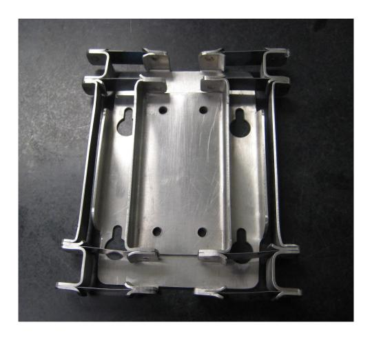
Note the curved edges of all parts touching the springs. Springs are spot welded.
