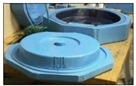
Both the catalyzed silicone rubber and the resin to be poured must be degassed by placing in a vacuum chamber for at least 30 minutes. Make sure the volume of the container is at least 5 times the volume of the liquid, as the liquid will foam up during degassing. Only
