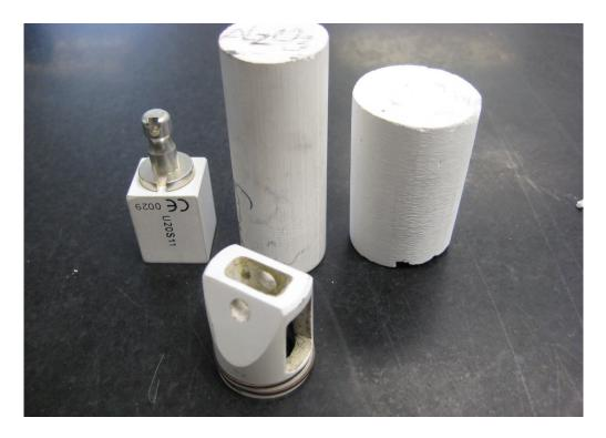
Machinable ceramics can be machined (before firing) with standard metalworking tools. Carbide tipped tools are preferred. Because of the abrasive dust they create during machining, a suction hose hooked up to a vacuum cleaner needs to be provided, as shown is the next photo:
