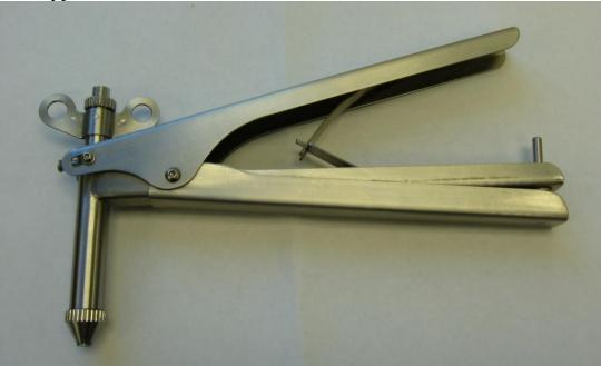
All parts except for the turned parts were done by WJ cutting, bending and spot welding. Total fabrication time (not including design) is about 8 hours.
