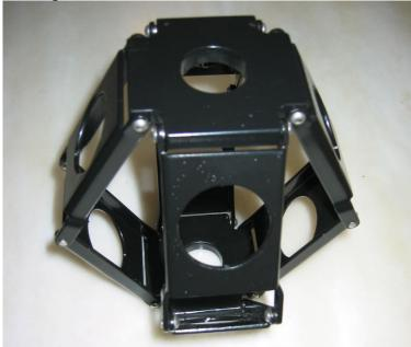
Simple linkage, 8 identical arms and two end pieces. Total fabrication time, including painting, is about 1 hour. Paint is fluidized bed Rilsan (acts as a bearing surface).
