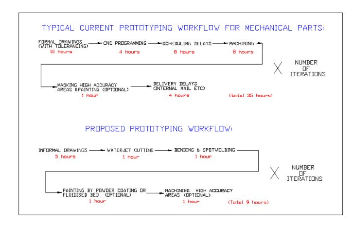
Another factor to keep in mind is that for simple parts the programming can be done in minutes right on the waterjet cutter, and the overall time from idea to part can be as fast as 10 minutes, for example a simple box or bracket. With traditional methods the time does not drop as dramatically as the CNC programming is rarely done on the machine and requites more care to avoid damaging the machine.
