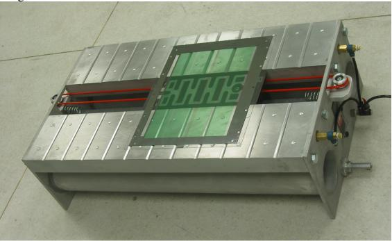
Proof-of-concept pressure/vacuum air bearing scanning table for a machine to manufacture LCD displays. Parts cut by WJ and assembled by adhesive bonding using a granite surface plate for alignment. Total fabrication time (including many parts not visible in photo) is about 12 hours.
