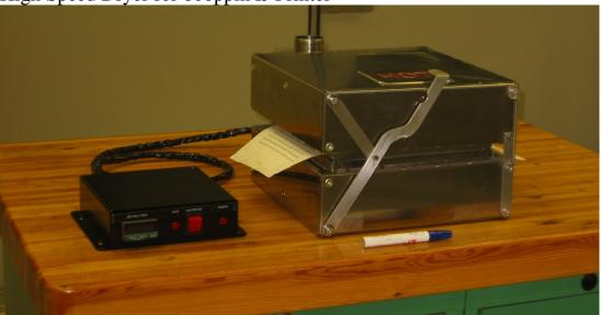
All parts of both dryer and control unit are WJ cut, bent and welded. No other machining used. Dryer is doubled walled with dual air bearing heat transfer.
