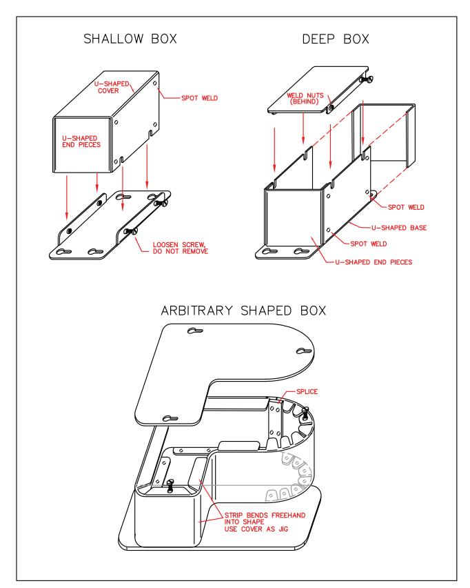
When making arbitrary shaped enclosures it is sufficient to bend the "wrap around" part in the form of a channel, all other bends can be done freehand as the channel will only bend where it is notched out. The radius of the bend id determined by the width of the notch, as can be seen below.
