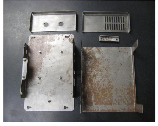
Before bending cover bend a test strip having the same length to check fit.
