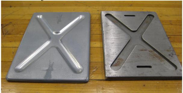
The tool to press the cover on the left is made of two layers, spot welded together. Total fabrication time for the tool and the cover is about 10 minutes. Pressed into hard polyurethane.
