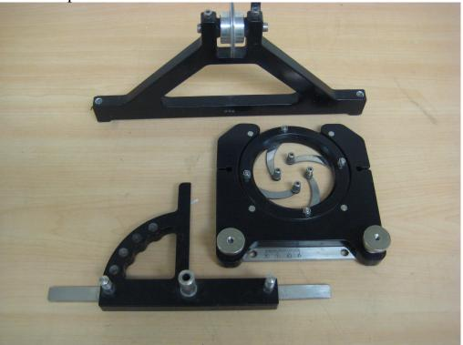
Cut from 12.7mm aluminum plate, painted, then machines at the critical areas. Total fabrication time 2-3 hours per part.
