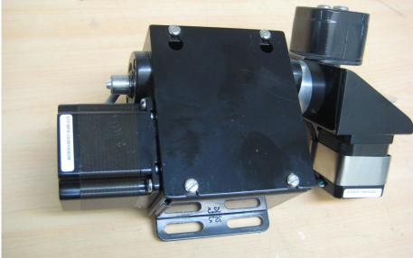
Assembly of stepper motors and gearbox based on timing belts. Shaft holes finish bored after painting.
