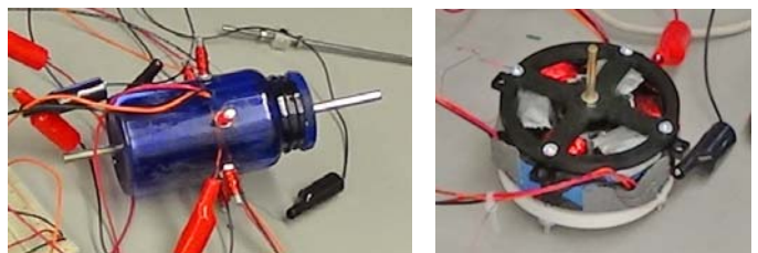
Fig. 3: Sample proof-of-concept and finished motor
