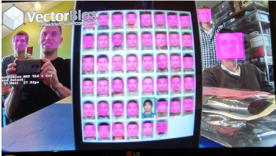
**Figure 3.7:** Photo of video output showing 49 of 50 faces detected on a 1080p image in 36 ms
