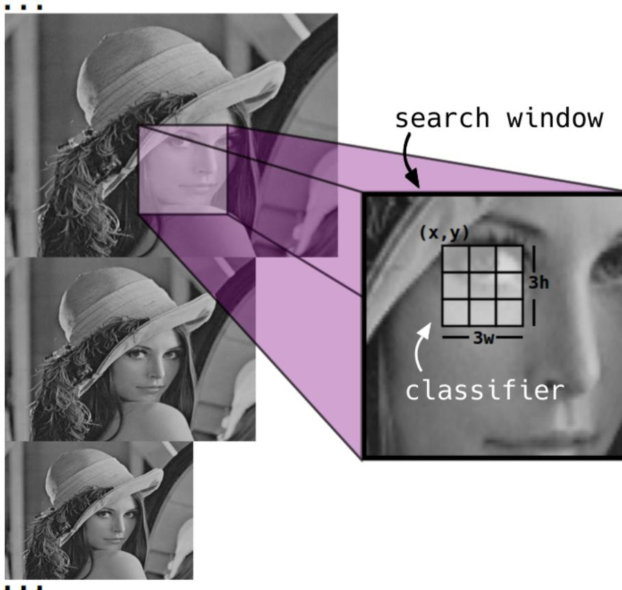
**Figure 2.1:** A search window traverses an image pyramid, evaluating a cascade of classifiers at each position.
