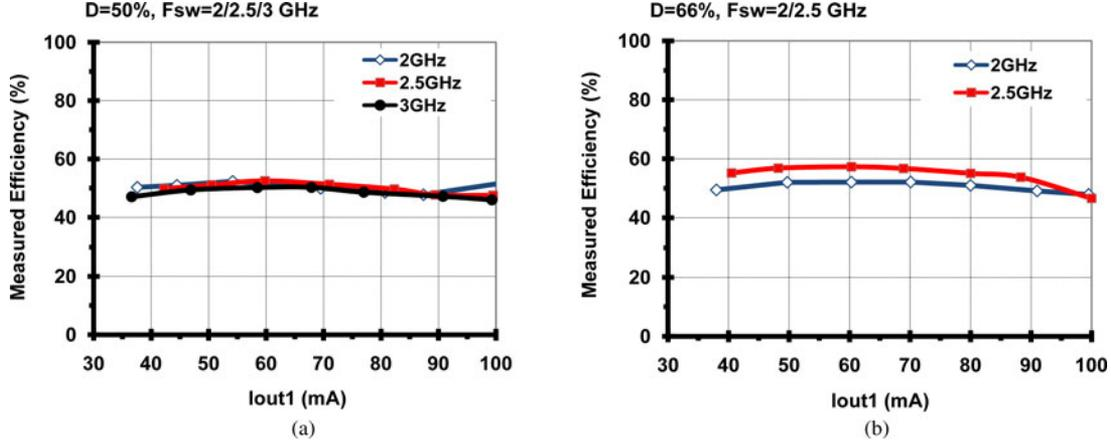
Fig. 14. Measured values of efficiency at different combinations of  $F_{sw}$  and  $D$  for the merged buck converter.
