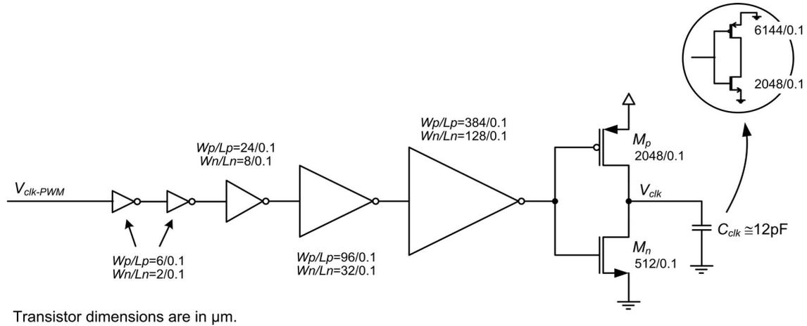
Fig. 5. Reference clock driver for the merged clock driver/buck converter.
