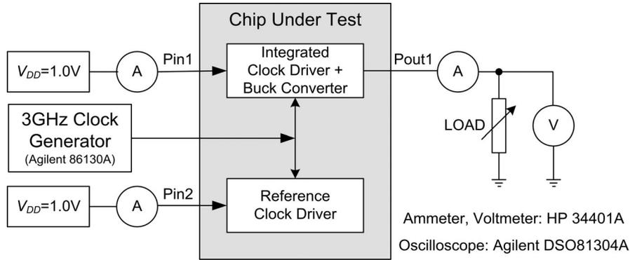
Fig. 11. Block diagram of the chip and test bench setup (four-point probing not shown).
