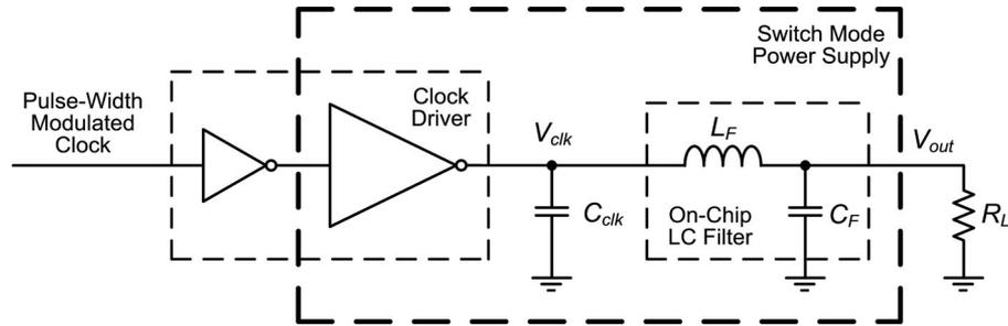
Fig. 1. Recycling clock energy with a dc–dc converter.
