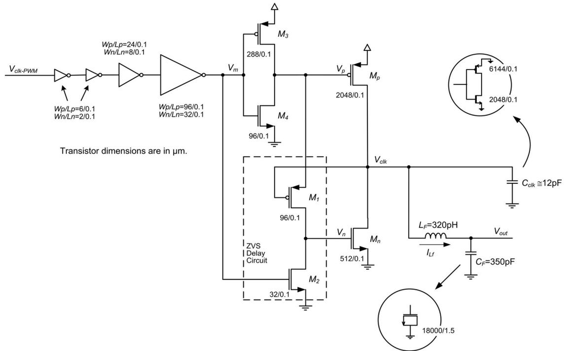
Fig. 6. Merged clock driver/buck converter.
