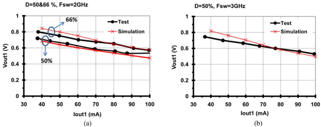
Fig. 12. Merged buck Converter: Output voltage  $V_{out1}$  in simulation, and measurement, at different combinations of  $F_{sw}$  and  $D$ .
