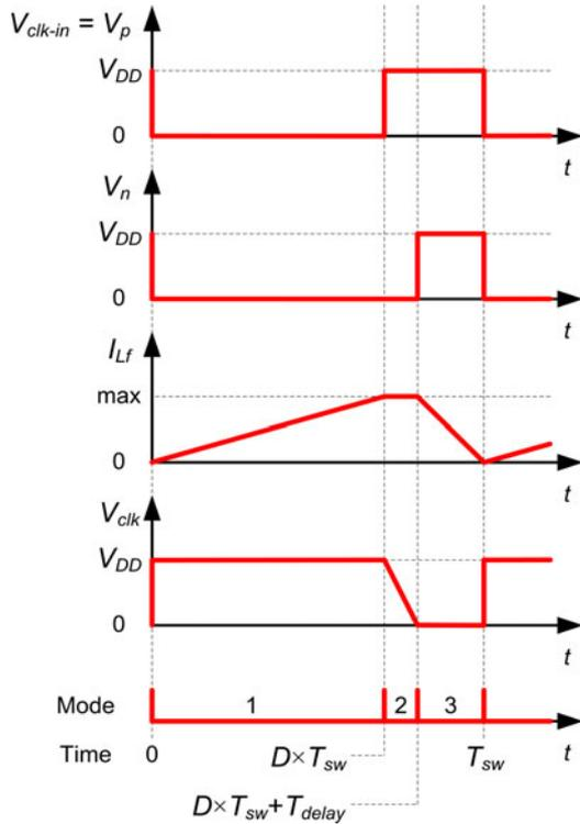
Fig. 4. Idealized timing diagrams for the merged clock driver/buck converter.
