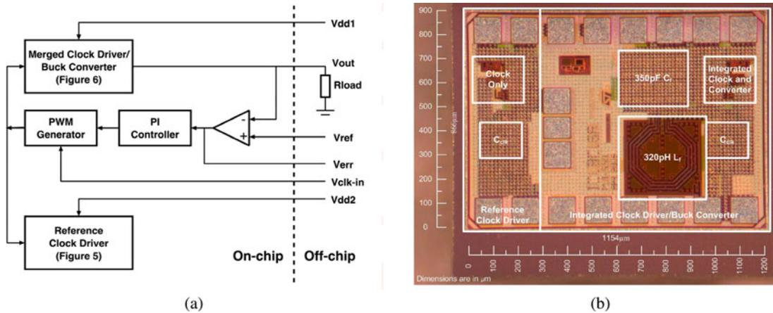
Fig. 7. (a) Block diagram and (b) chip micrograph of fabricated design.
