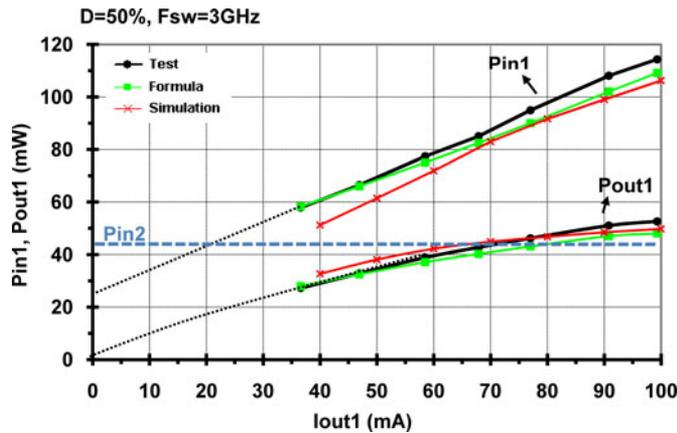
Fig. 13. Evaluating power values of  $P_{in1}$ ,  $P_{in2}$ , and  $P_{out1}$  in simulation, calculation, and measurement, at (3 GHz, 50%).
