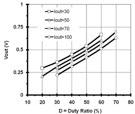
Fig. 9. Simulation results of the merged clock driver/buck converter: Output voltage versus duty cycle.
