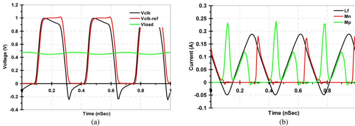
Fig. 8. Simulated waveforms of points of interest for the merged clock driver/buck converter. (a) Voltage waveforms. (b) Current waveforms.
