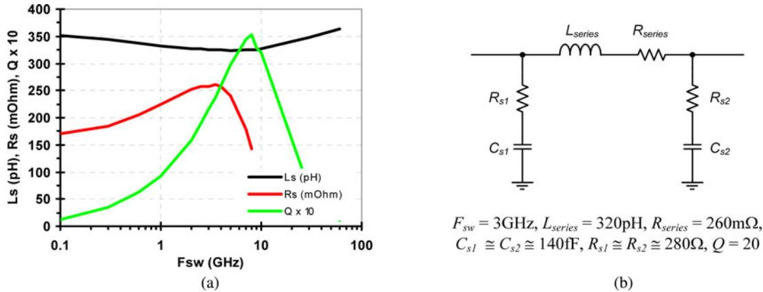
Fig. 10. Modeling of the on-chip inductor for the buck converter chip. (a)  $L_{series}$ ,  $R_{series}$ , and  $Q$  versus  $F_{sw}$ . (b) Simplified  $\pi$  model.
