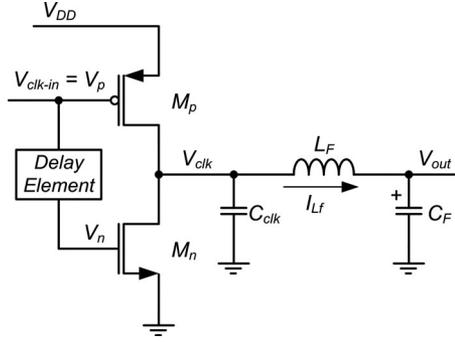
Fig. 3. Simple merged clock drive/buck converter.
