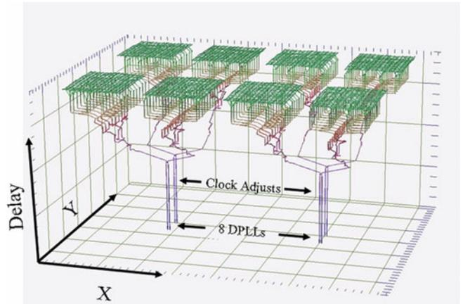
Fig. 2. IBM POWER7 clock network [1].
