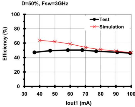
Fig. 15. Merged buck converter: Measured versus simulation.
