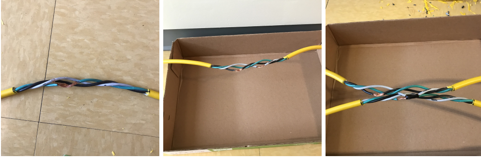
Fig. 6: Photos of applied degradations (Left) at Spot B after execution of Stage 3, (Middle) at Spot A after execution of Stage 5, (Right) after execution of Stage 7.
