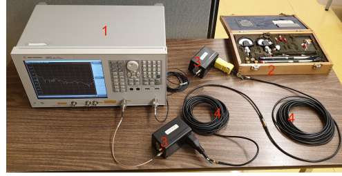
Fig. 2: Illustration of the measurement and calibration setup. (a) Schematics for DUT and ancillary components. (b) Photo of the calibration setup (through measurement). Labelled items are 1—VNA, 2—calibration kit, 3—couplers, 4—connection cables.
