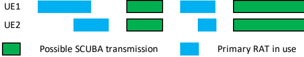
Fig. 3. An illustration of the TDM nature of SCUBA, which operates as a secondary RAT only when both devices are idle in their primary RATs.
