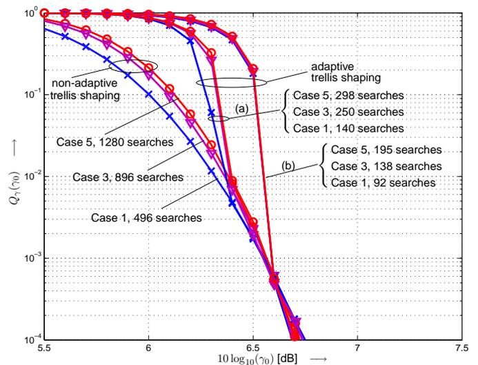
Fig. 3. Performance of non-adaptive and adaptive trellis shaping and the number of searches required. (a) Threshold chosen as the 1% PAR. (b) Threshold chosen as the 0.1% PAR. VA with Metric 2. Cases 1, 3, and 5 from Table I.
