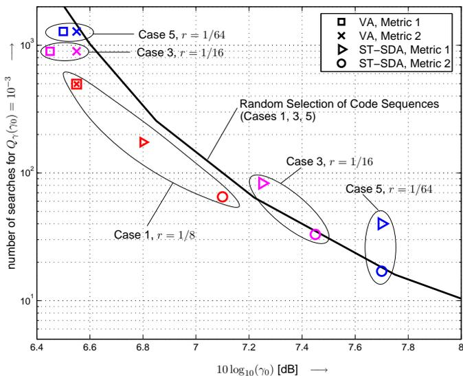
Fig. 2. Performance of trellis shaping, VA and ST-SDA with Metrics 1 and 2, respectively. Cases 1, 3, and 5 from Table I. Also shown: Random selection of code sequences (SLM-like PAR reduction).
