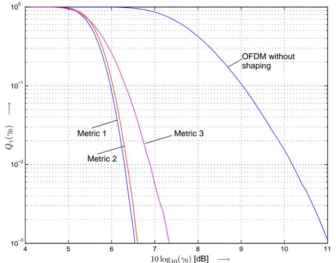
Fig. 1. Performance of trellis shaping with VA and Metrics 1-3. Case 1 from Table I.
