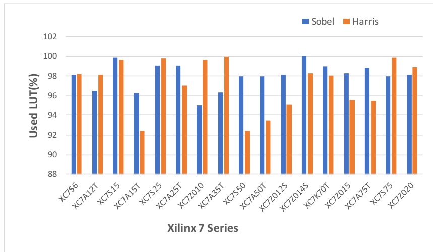
Figure 4.16: Percentage of LUT usage for different Xilinx FPGAs
