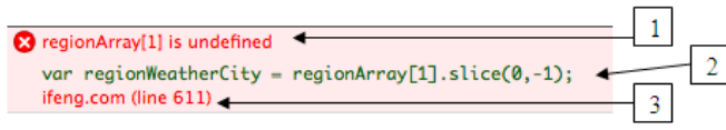
Fig. 1: A screenshot of a JavaScript error message as shown in the Firebug error console. The error message consists of (1) the text description, (2) the line where the error occurred, and (3) the JavaScript file containing the erroneous line.
