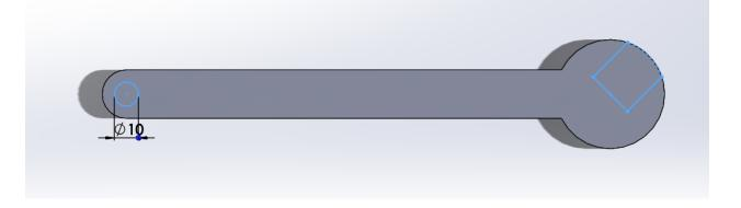
To sketch the shape on the right, simply start with a circle that is identical in shape and size to the original circle. Next, select the 3 Point Center Rectangle tool (click the small triangle next to the rectangle tool to access more options).
