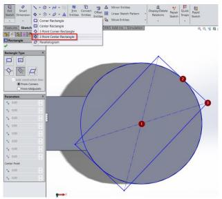
Now set the width of the rectangle to 20mm (to fit our hex nut from the previous example). Afterwards, set the angle of the rectangle to  $45^{\circ}$  by selecting one of the longer sides and choosing  $45^{\circ}$  in the parameters panel on the right.
