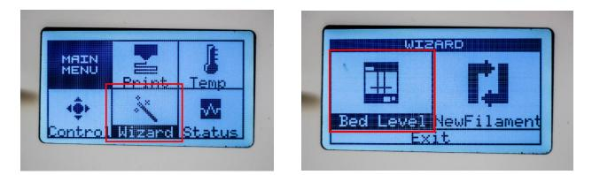
Follow the instructions on the display, ensuring that a small space is left between the printer head and the build platform at every point (about 1mm or less). To change the distance between the printing bed and the printing head, adjust the small black dials on the bottom of the bed.
