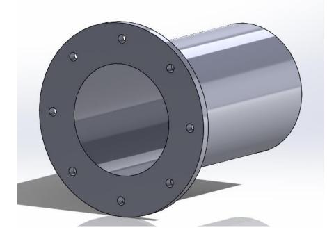
5. The next step is to mirror this part so we have a full length section of pipe with bases at either end. To do this we will use the Mirror tool in the features tab. Select the mirror tool, then select the face without the base as the Mirror Face/Plane. In the drop-down menu on the left side, select all 4 features as the Features to Mirror.
