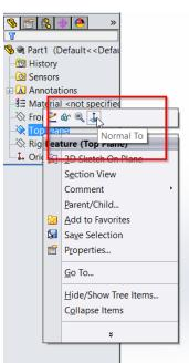
3. While the Top Plane is selected, switch to the Sketch tab at the top of the interface and select the "Sketch" tool in the top left corner. We are now creating a sketch on the Top Plane. Anything we sketch will appear on the Top Plane.
