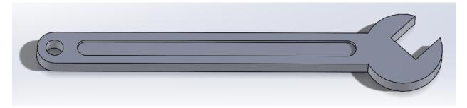
6. Fillets are crucial when considering the mechanical properties of a part. Fillets reduce stress concentrations, eliminate dangerous sharp edges, and make the part more ergonomic.
