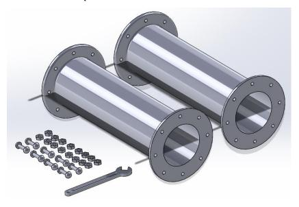
6. Once we have the correct number of parts we are ready to assemble our pipeline. It is helpful to fix one of the pipe sections so it doesn't move, and attach all the other parts to the one fixed pipe section. Right click one of the pipe sections in the panel on the left and click fix.
