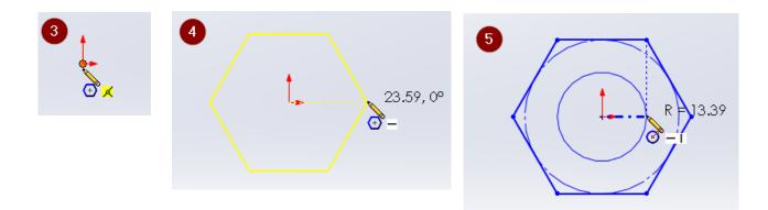
4. Now we will assign dimensions to our outline. Make sure we are still in sketch mode by looking at the top left corner and seeing that the Sketch button is depressed and now reads "Exit Sketch". Press the "S" key on the keyboard. In the small window, click the "Smart Dimension" tool.
