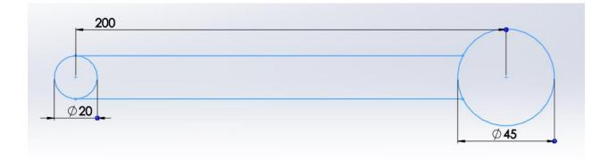
2. Make sure this sketch is selected and use the extrude tool to extrude this shape by 10mm. We now have our basic wrench shape. From this part we will cut away pieces and round edges to obtain our final product. NOTE: you will have to select all 3 contours when extruding this shape, otherwise only one region of the wrench will be extruded.
