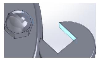
Finally, mate the bottom curve of the wrench head to the corresponding side of the nut. The wrench should now be fully mated to the nut. The assembly at this point is finished.
