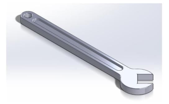
1. First, start a new part and sketch the shapes below on the top plane according to the given dimensions. NOTE: the lines are tangent to the top and bottom of the smaller circle.
