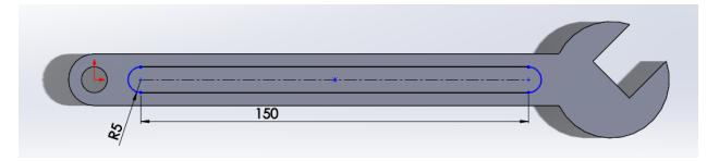
Extrude Cut this sketch down, but not all the way through. Cut 2.5mm into the part. At this point our wrench is almost done, the only thing left to do is fillet the edges.
