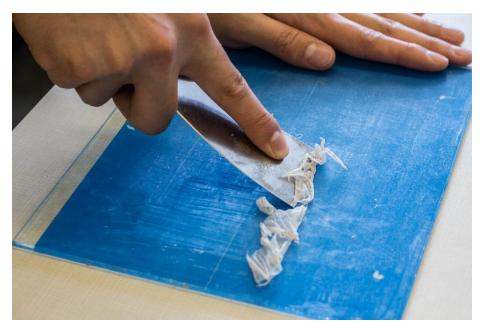
Be sure to use the glass panes provided as the build platform, never print directly on the printing tray of the Tinkerine Ditto Pro. Once the built platform is clean, apply glue over the surface of the build platform. The glue will ensure that the filament sticks to the build platform.
