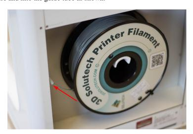
Press the tensioner button down to thread the new filament into the hot end of the printer head.
