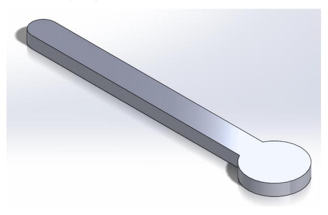
3. Now make a sketch on the top surface of the wrench, instead of making a sketch on the top plane, as we have done so far. Simply right click on the top surface of the wrench and click the sketch tool. Sketch the shapes as shown below, starting with the circle on the left.
