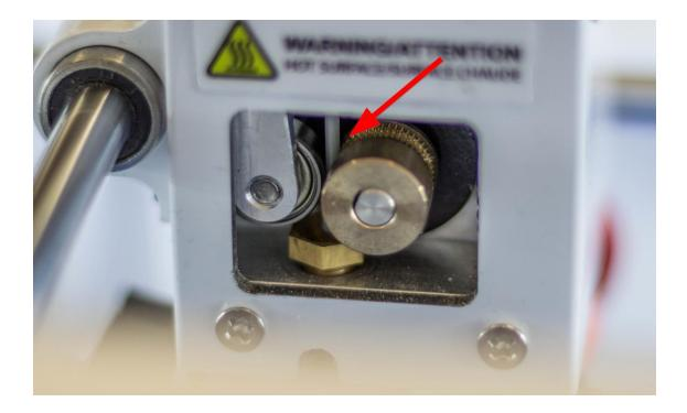
Push the filament through the head until it comes out of the hot end. Trim off the excess filament. If the printer was previously loaded with a different colored filament, push the new filament through until you see the new color come out of the hot end.
