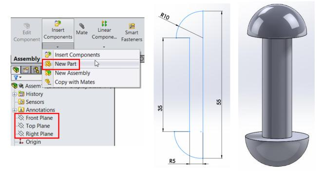
5. Once the pin is designed within the assembly we have all parts necessary to construct our pipeline! One of each part should already be in the assembly from step 2. To copy parts, simply click and drag a box around the part you wish to copy until the entire part turns blue, and CTRL + C and CTRL + V as many copies as needed. For this assembly we will need 2 of the pipe section, 16 hex nuts, 1 wrench and 8 pins.
