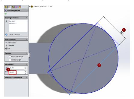
At this point the center of the rectangle may have shifted. If this is the case, simply select both the center of the rectangle and the center of the circle (CTRL + left click) and selecting Midpoint in the Add Relations panel on the left side.
