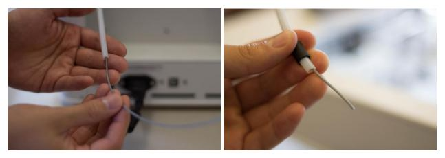
Ensure that the spool is hung neatly on the back of the printer, with the filament being spooled out clockwise and into the guide tube as shown.
