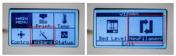
Remove any old filament and feed the new filament up through the guide tube and out the other side.
