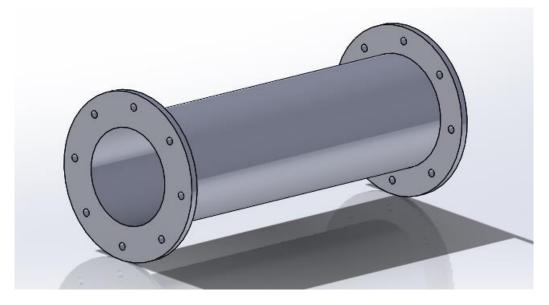
In this instance we can simply shell the mirrored section again to achieve the hollow inside.
