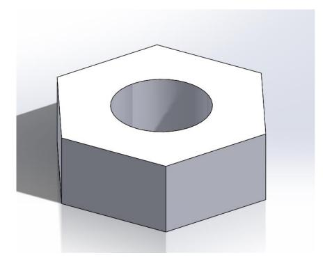
6. At this point we are done drafting our first simple part. Hold down the middle mouse button and move the mouse around to view different angles of the part. Hold CTRL+middle mouse button and move around to pan. Scrolling the middle mouse button will zoom in and out. Save this part as a \*.prt;\*.sldprt file. We will be using this part in later tutorials.
