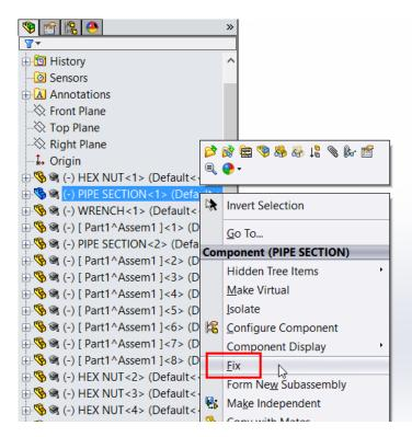
7. Once one of the pipe sections is fixed we are ready to mate the other components to it. Mating is a tool used in assemblies to attach components together.
