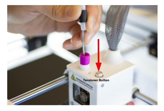
Note the position of the filament, make sure it is fed in between both gears.
