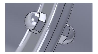
10. Repeat this process for all 8 bores, using all 16 nuts and 8 pins in the process. The assembly should appear as follows. Take note: the nuts and pins are still able to rotate freely. It is possible but not required to apply a lock mate (under standard mates) to the nuts and any surface of the pipe section to ensure that they are not free to rotate.
