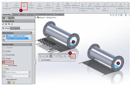
Note how SolidWorks recognizes the surfaces to be mated and automatically selects the Concentric Mate. There are many different mates as seen in the Standard Mates panel. In addition to the standard ones, there are Advanced Mates and Mechanical Mates, which are more complex and have more parameters.
