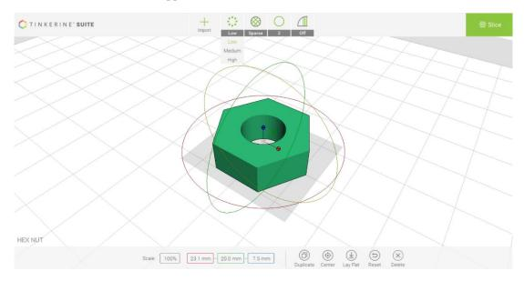
4. The resolution parameter controls the accuracy and precision of the printed material. The higher the resolution, the more precise the printing will be.
