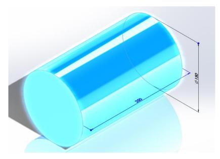
2. Next, use the Shell tool to hollow out the inside of this cylinder. The Shell tool is found in the features tab. Select the Shell tool, click both the circular faces for the Faces to Remove and set the Thickness to 10mm.
