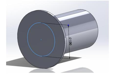
Next, we will use the Circular Sketch Pattern to sketch a series of circles around the outside of the base. First add a circle at the top of the base, 10mm in diameter and 94mm from the center.
