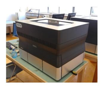
These are two 3D printing technologies are fundamentally different and as such, they are both different in terms of material used, cost, functionality, etc. The Tinkerine DITTO PRO 3D printer has a lower absolute resolution, is much cheaper (both the cost of the printer and the build material), and can print parts much quicker. The Objet printers are able to achieve much higher precision and resolution, but cost considerably more and are also much slower in printing parts.
