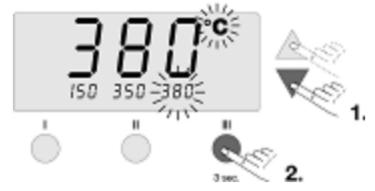
Setting a Radio Button to a low temperature gives you the option of manually and quickly decreasing temperature when the soldering iron is not being used.
