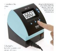
By depressing a Radio Button, the pre-selected value for that button now becomes the "Set" temperature. The new value appears for approximatly 2 seconds in the display and the temperature symbol flashes **°F** (or **°C**). The display then switches back automatically to the "Read" value.
