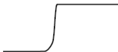
Signal with a short length ground lead
