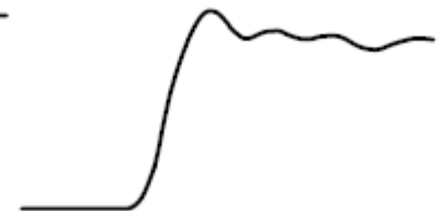
Signal with a long ground lead
