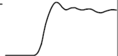
Signal with a long ground lead
