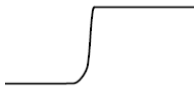
Signal with a short length ground lead
