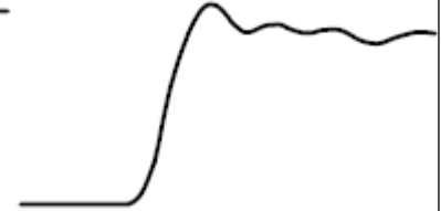
Signal with a long ground lead
