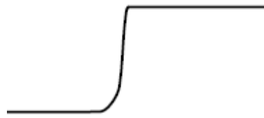
Signal with a short length ground lead
