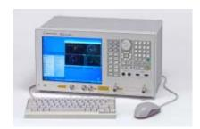
The E5061B help provides an easy access to the information related to the use of Agilent E5061B Network Analyzer. Pressing Help key on the front panel displays the topic related to the selected softkey.
