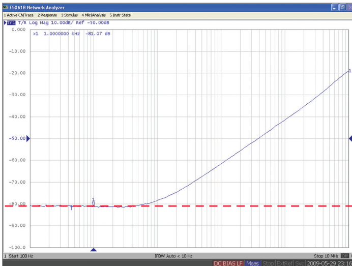
OP-amp PSRR measurement (100 Hz to 10 MHz)
