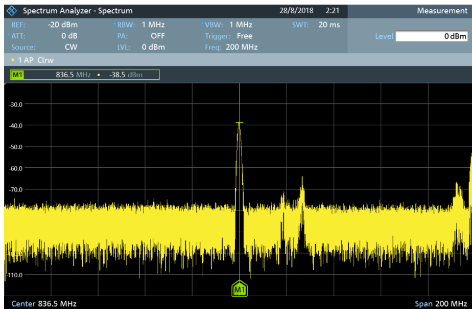
Figure 9.3: Example of measuring the received power
