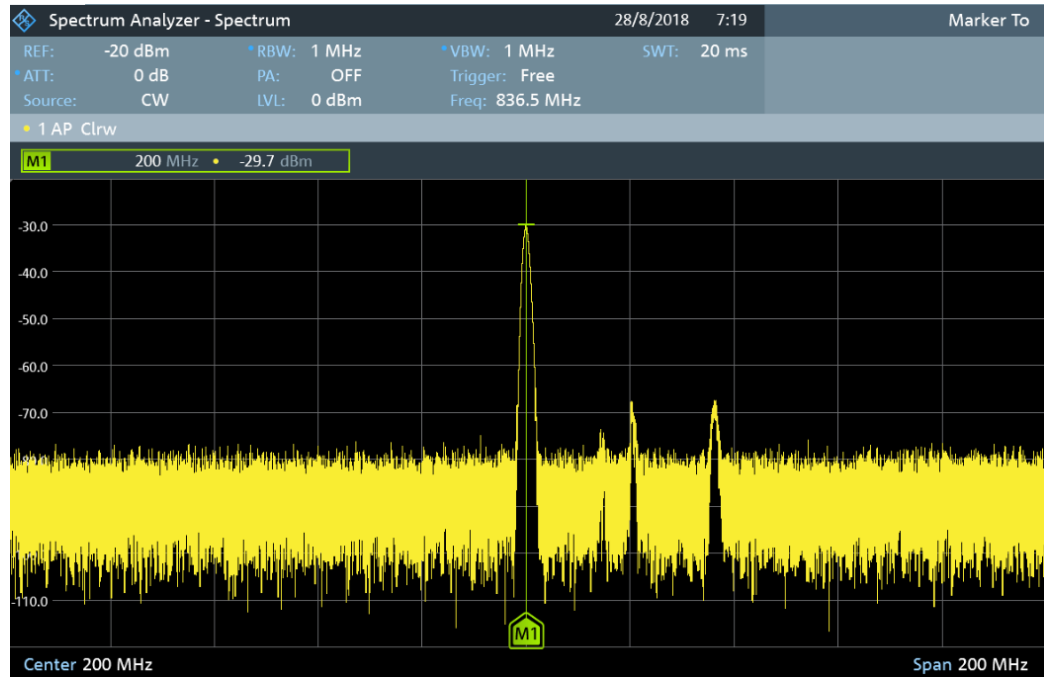
Figure 9.6: Example of measuring the received power
