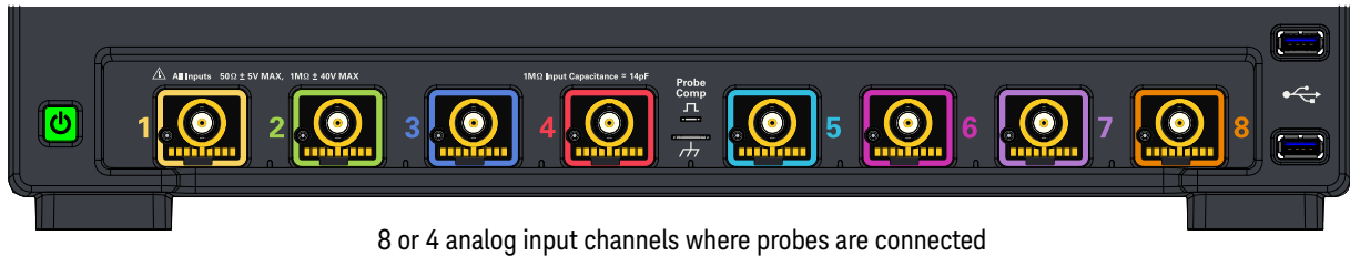
Figure 9 MXR/EXR-Series oscilloscope probe connectors
