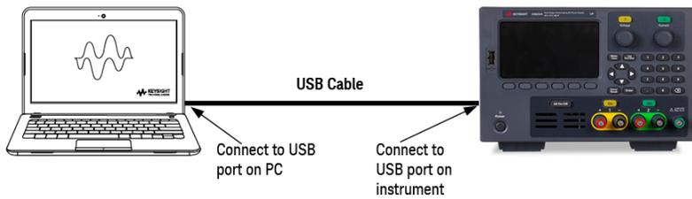
1. Connect your instrument to the USB port on your computer using a USB cable.
