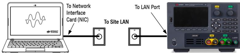
1. Connect the instrument to the site LAN or to your computer using a LAN cable. The as-shipped instrument LAN settings are configured to automatically obtain an IP address from the network using a DHCP server (DHCP is ON by default). The DHCP server will register the instrument's hostname with the dynamic DNS server. The hostname as well as the IP address can then be used to communicate with the instrument. The front panel **LAN** indicator will come on when the LAN port has been configured.
