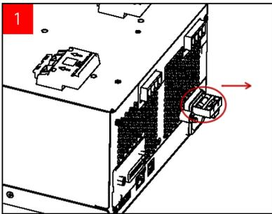
Turn the unit around and place it on a hard, flat surface with its rubber feet up. Locate the fuse holder as shown in the image above, and pull the fuse holder out of the power supply.
