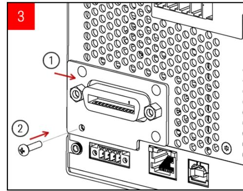
Put the module into the unit and slide the GPIB board to the right so that it is flushed against the instrument's sheet metal. Use the screw that was removed earlier to secure the GPIB plate in place.
