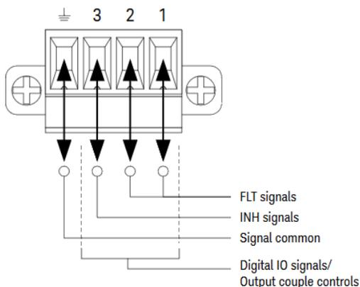
The digital I/O pin can be used to control both relay circuits as well as digital interface circuits. The figure above illustrates typical relay circuits as well as digital interface circuit connections using the digital I/O functions.
