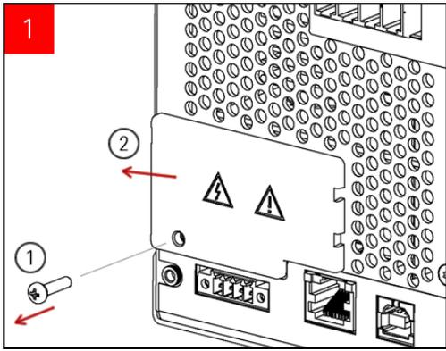
Use Phillips head screwdriver to remove the screw from the GPIB cover plate. Retain the screw for use later in this procedure.
