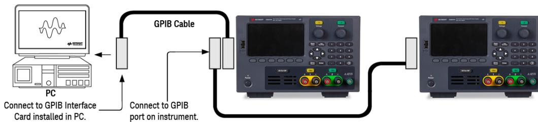
1. If you do not have a GPIB interface card installed on your computer, turn off your computer and install the GPIB card.
