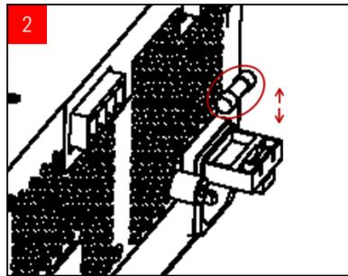
Remove the blown fuse and insert the proper replacement fuse into the fuse holder.
