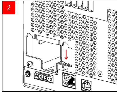
Locate the connector, just inside the unit, to connect the cable that is attached to the GPIB module.
