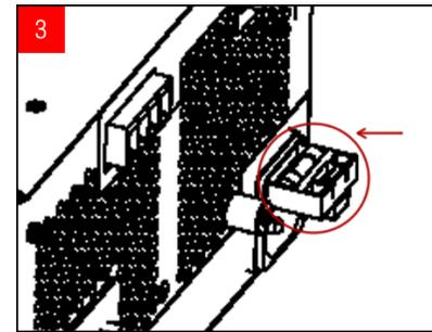
Re-insert the fuse holder into the power supply. Place the unit back to its proper orientation.
