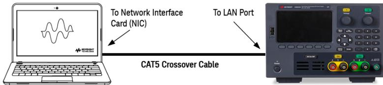
1. Connect the instrument to the computer using a LAN crossover cable. Alternatively, connect the computer and the instrument to a standalone hub or switch using regular LAN cables.
