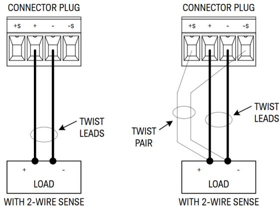
Connect the load to the output terminals using separate connecting wires. Keep the wire-pair as short as possible and twist or bundle it to reduce lead inductance and noise pickup. Keep the load leads under 14.7 meters (50 feet) per lead because of inductance effects.
