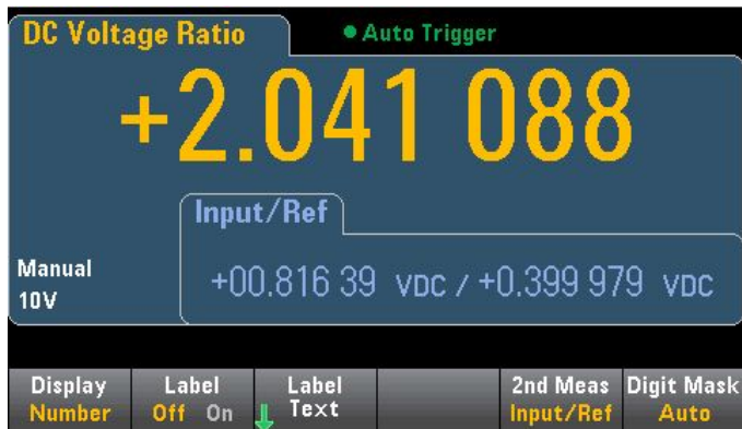
Figure 7. With the Truevolt DMM dual display, you can view two voltage measurements when using the DCV ratio function
