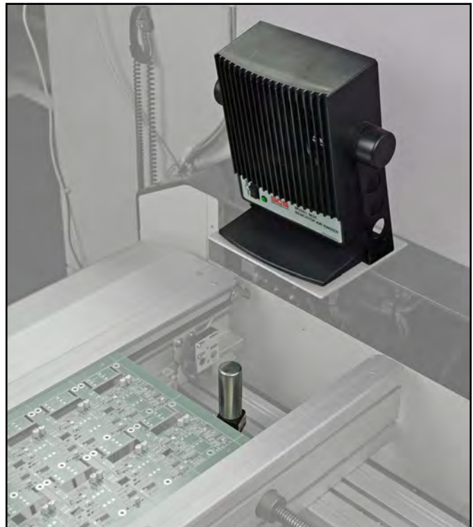
Figure 23. Using the EM Aware Monitor with ionizer antenna on an SMT conveyor with the SCS 963E Benchtop Air Ionizer
