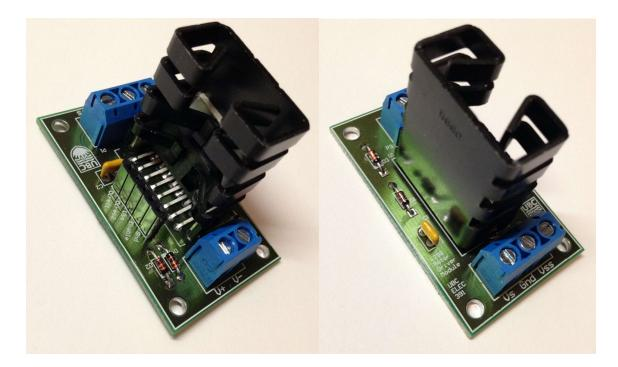
This board features the L298 Motor Driver IC. The dual channels of the L298 have been tied together to create a simple single channel motor driver.
