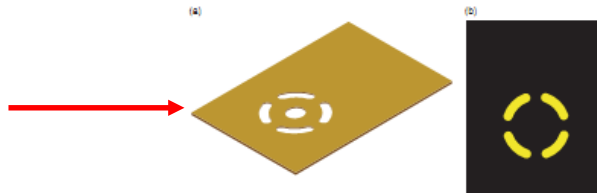
Figure 1-18 Copper in a plane layer (negative view without drill info). (a) Copper plane with thermal relief. (b) Negative view in Layout.
