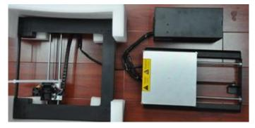
4. Cut the white ribbon that secures the Extruder Assembly to the Tower Frame.
