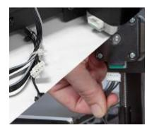
13. Mate the two-pin black cable connector in the cable bundle with the corresponding black connector on the cable attached to the stop switch.
