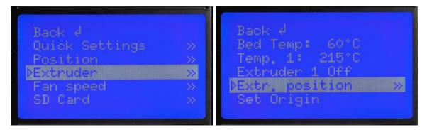
26. Insert the included MicroSD card into the slot on the side of the Power Supply, then select SD Card > Mount Card. Finally, select SD Card > Print File, select one of the sample 3D model files, then press the knob to start printing.
