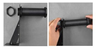
11. You can mount the **Filament Stand** and **Spool Holder** onto either the **Tower Frame** or the **Power Supply/Control Box**. Use two hex and the hex wrench to secure it to your desired location. If mounting it to the tower frame, ensure that the spool holder is mounted over the center of the tower frame.
