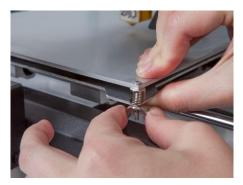
21. Now that the printer is off you can manually move the extruder around the build platform. Because most printing is done near the center of the platform, you should check the nozzle height at points about 2 inches from each corner, as indicated by the blue X marks in the diagram below.
