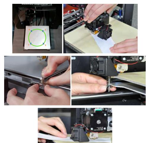
22. Switch the printer on and wait for it to initialize. Select **Position > Z. Pos. Fast**, then turn the knob to raise the extruder so that it is at least an inch above the build plate.
