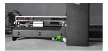
Open the accessories box and remove four Hex Screws and the Hex Wrench. Insert a screw into hole on the frame on the left side and tighten it using the hex wrench. Repeat the process on the right side.
