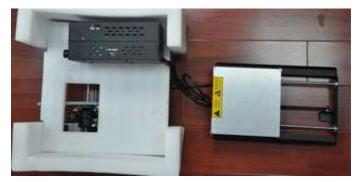
3. Remove the **Power Supply/Control Box** and place it next to the base.
