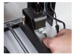
15. Insert the white connector on the short cable on the right side of the base into the corresponding white connector of the right side Z-axis stepper motor.
