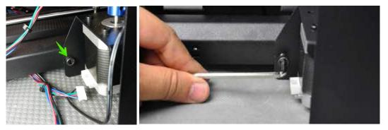
8. Flip the printer onto its left side, then insert a screw from inside the base and secure it to the frame using the hex wrench. Flip the printer onto the other side and repeat the process.
