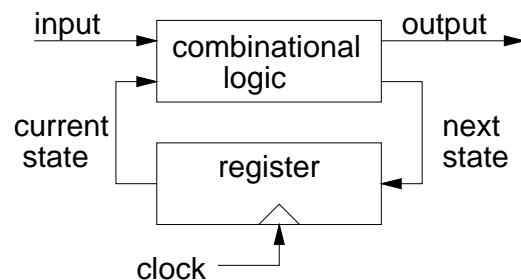
State machines in VHDL are implemented by using selected or conditional assignments to compute output and next state from the current state and the inputs. A process is used to implement the register that defines the current state.
