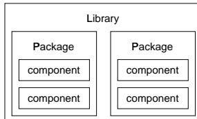
To save component declarations we put them within a package declaration. When this file is compiled ("analyzed") the information about the components in the package is saved in a file. The components in the package can then be used in other designs by making them visible with a `use` statement.
