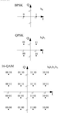
QAM modulation with M symbols is known as M-QAM, for example 16-QAM, 256-QAM, etc. The constellations for M = 2 and M = 4 are the same as those for BPSK and QPSK modulation as explained below. Values of M from 2 up to 1024 (10 bits per symbol) or even more are used. Higher values of M are used on channels with low levels of noise and distortion.
