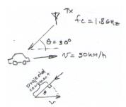
**Exercise 1**: A receiver in a car receives a 1.8 GHz signal while travelling on a road at 50 km/h. The road is at an angle of 30 degrees relative to the direction of arrival of the signal. What is the velocity relative the direction of arrival of the signal? By how much does the path length change each second in meters? In wavelengths? What is the Doppler shift?
