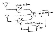
Adaptive antenna arrays are sometimes called "smart antennas" or "phased arrays".
