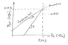
The power at which the third-order component would have the same power as the fundamental is called the third order intercept point (IP3). This can be an input power (IIP3) or output power (OIP3). The two are related by the gain of the amplifier.
