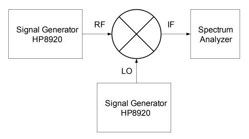
From the datasheet, what is the LO power required for this mixer? Measure the mixer output at 100 MHz using the Spectrum analyzer, using different LO power levels (LO power = -6 dBm, 0 dBm, +6 dBm). Record the mixer output power in each case, and compute the conversion loss. <u>How does the conversion loss compare to the datasheet value?</u> What happens to the conversion loss as the LO power is reduced?
