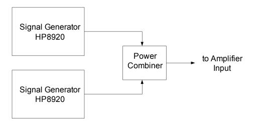
Apply the 2-tone signal to the amplifier input, and measure the amplifier output using the Spectrum Analyzer. Make a sketch of the output spectrum, noting the frequency components and the power levels. <u>Identify the intermodulation products, and calculate the Input IP3 (IIP3) and Output IIP3 (OIP3) for this amplifier</u>. Compare your measurements against the amplifier's datasheet, and comment on the results.
