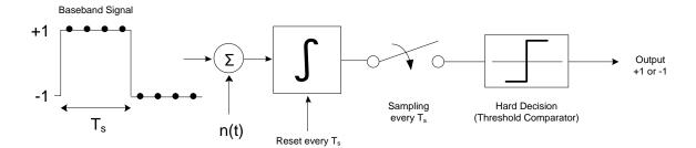
In this receiver, the signal is integrated over each symbol period. At the end of each symbol period, the sum is then passed into the threshold block to decide whether the received symbol is +1 or -1. For the next symbol period, and result from the previous symbol period is dumped by resetting the integrator back to zero.
