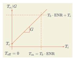
The noise source outputs a noise level defined by its "excess noise ratio" (ENR) =  $T_{on}/T_0$ . Since the noise source and amplifier-generated noise are independent, their powers will add and it's possible to solve for  $T_e$  and F.
