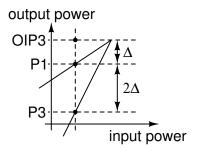
Thus measuring the output level, P1 (dBm) and the relative level of the third-order product,  $2\Delta = P1 - P3$  (dB) allows us to compute OIP3 as  $P1 + \Delta$ . However, these measurements must be made in the region where P1 is increasing linearly with the input power.
