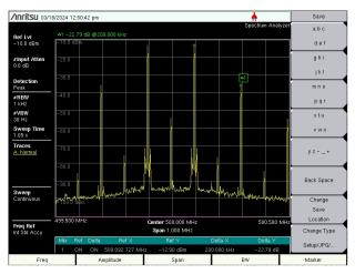
To measure the levels of the intermod products, set a marker on one tone and measure the difference to the IM3 product using the following menu items:
