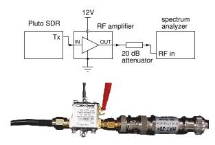
Connect the Pluto SDR TX output to the IN port of the amplifier using the short SMA-to-SMA cable included in the kit. Connect the amplifier's OUT port to a 20 dB attenuator using an SMA-to-BNC adapter. Connect the attenuator to the spectrum analyzer with a BNC cable.
