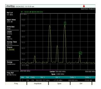
To measure the levels of the intermod products, set a marker on one tone and measure the difference to the IM3 product using the following menu items:
