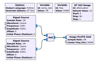
The complex signal sources have amplitudes of 0.5 and frequencies of +100 kHz and -100 kHz:
