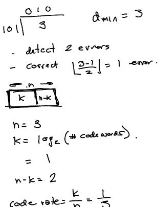
**Exercise 3**: How many errors can an *N*-fold repetition code detect? Correct? What is the code rate?
