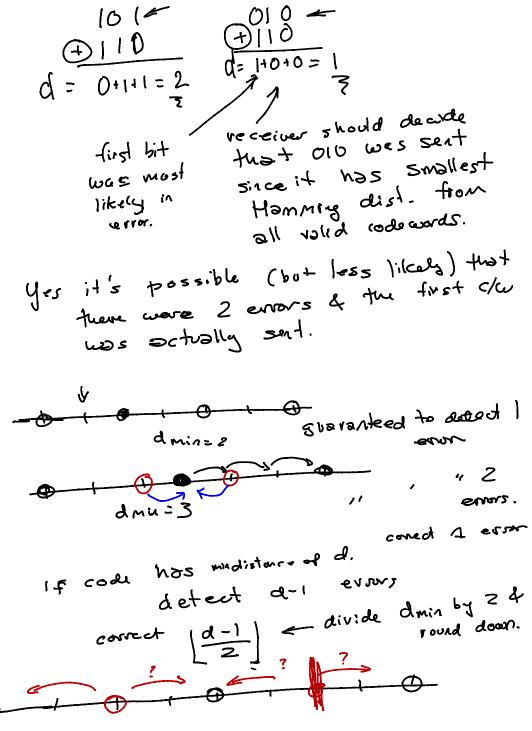
**Exercise 2**: What is the minimum distance for the code in the previous exercise? How many errors can be detected if you use this code? How many can be corrected? What are n, k, and the code rate (k/n)?
