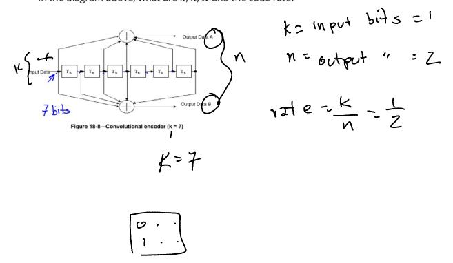
**Exercise 14**: Consider the convolutional encoder above. If the only the bits corresponding to the outputs A, A and B, and B are transmitted corresponding to every three input bits, what is the code rate of this punctured code?
