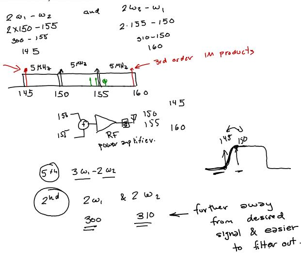
**Exercise 2**: An amplifier has an OIP3 of 30dBm. If it is required that the adjacent channel power be 30dB below the in-channel power, what is the maximum output power we should try to get from this amplifier?
