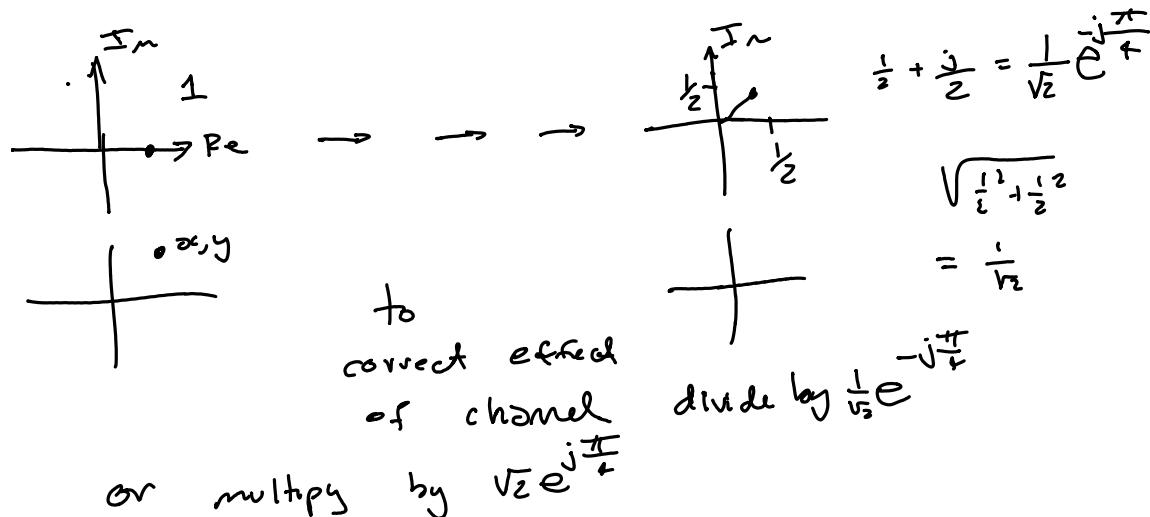
In general, if channel multiplies a pilot tone by  $X$ , we multiply the data on that subcarrier by  $X^{-1}$  (multiply by  $\frac{1}{|X|}e^{-j\angle X}$ ).
