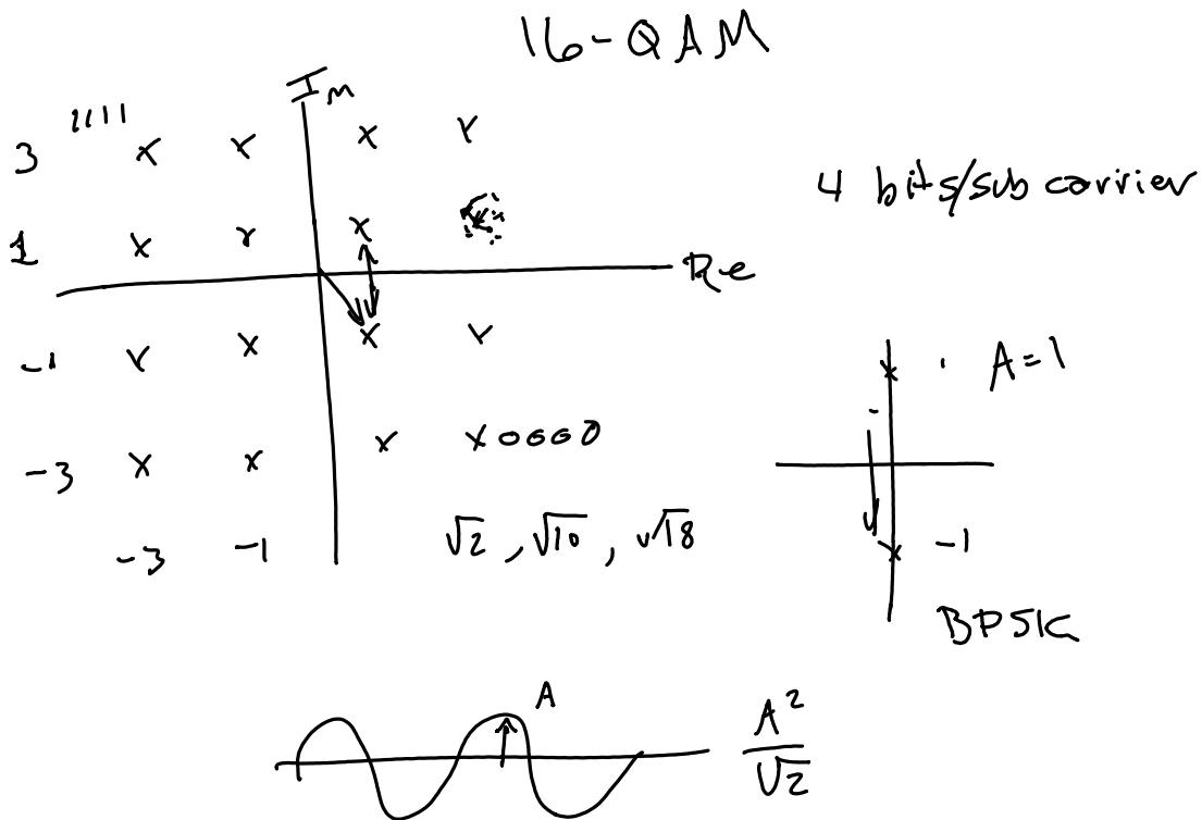
Note: this is the power of each subcarrier, not of the OFDM signal. The total power is the sum of the subcarrier powers (assuming independent modulation).
